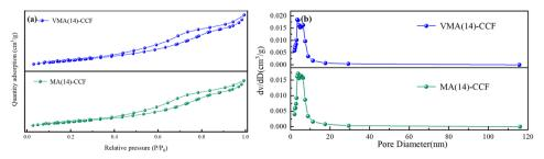
Fig. 5 N<sub>2</sub> absorption and desorption curves and pore size distribution of VMA(14)-CCF and MA(14)-CCF.
