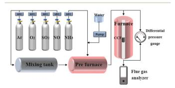
Fig. 1 Experimental device diagram.
