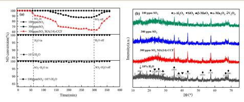
Fig. 7 (a) NO conversion and (b) XRD spectrum of VMA(14)-CCF and MA(14)-CCF in the presence of SO<sub>2</sub> and H<sub>2</sub>O at 225 °C.
