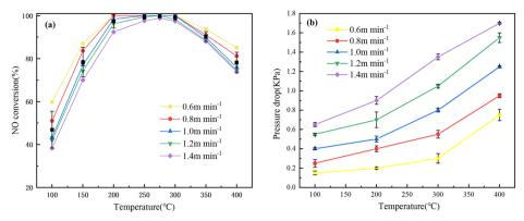
Fig. 6 (a) NO conversion and (b) Pressure drop of VMA(14)-CCF with different FV.
