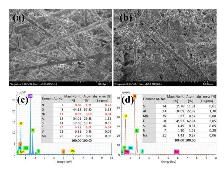
(a) SEM and EDS of VMA(14)-CCF and MA(14)-CCF after 300 ppm SO<sub>2</sub> at 225 °C.
