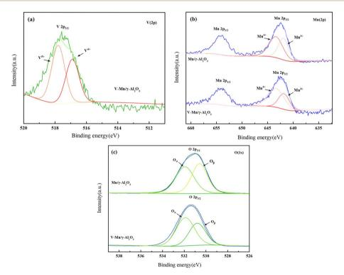
Fig. 4 XPS spectra of Mn/ $\gamma$ -Al<sub>2</sub>O<sub>3</sub> and V-Mn/ $\gamma$ -Al<sub>2</sub>O<sub>3</sub>.
