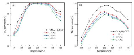
NO conversion of (a) VMA(14)-CCF and (b) MA(14)-CCF in the presence of Na.
