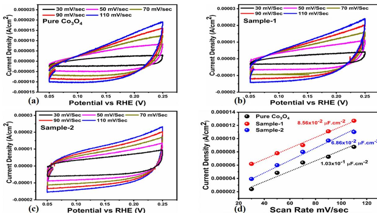
Fig. 7 (a–c) Non-faradic CV scans at different scan rates for pure  $Co_3O_4$ , sample 1 and sample 2 in an electrolyte solution of 1.0 M KOH. (d) Calculated ECSA values of pure  $Co_3O_4$ , sample 1 and sample 2.
