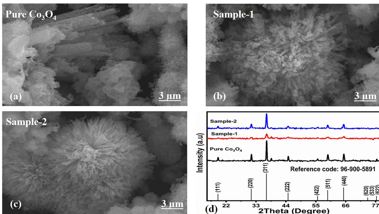
Fig. 1 (a–c) Prominent SEM images of different samples including pure  $\text{Co}_3\text{O}_4$ , sample 1 and sample 2. (d) XRD reflection peaks of pure  $\text{Co}_3\text{O}_4$ , sample 1 and sample 2.
