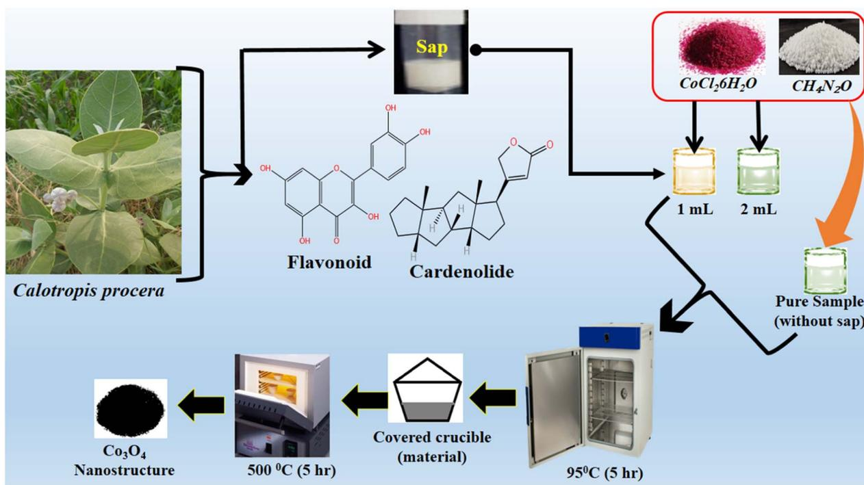
Scheme 2 Stepwise preparation of  $\text{Co}_3\text{O}_4$  nanostructures with the milky sap of CP.
