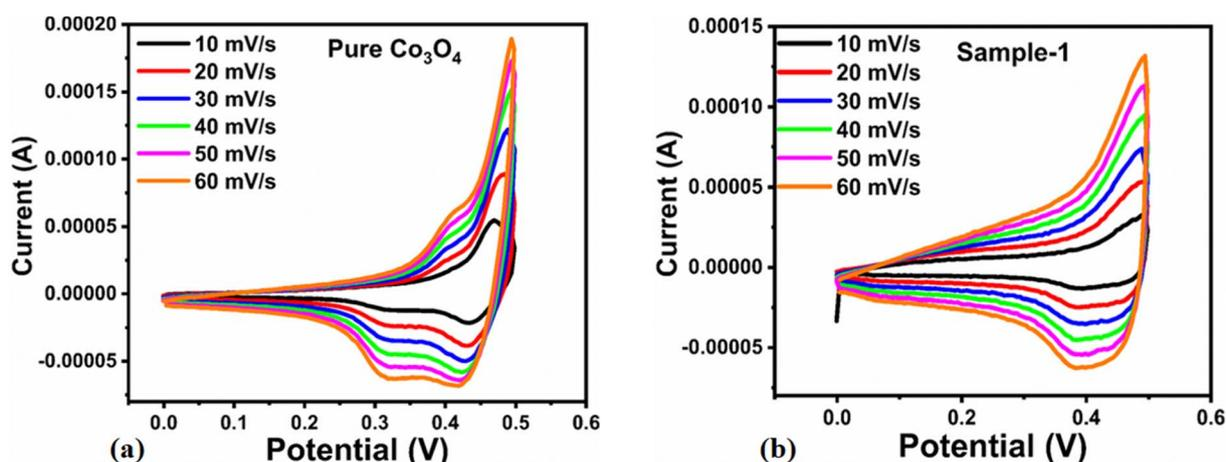
Fig. 8 (a) CV scans of pure  $\text{Co}_3\text{O}_4$ . (b) CV scans of sample 1 at different scan rates in 3.0 M KOH to describe capacitance properties.
