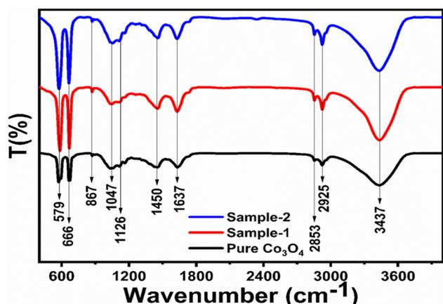
Fig. 4 FTIR spectra of pure  $\text{Co}_3\text{O}_4$ , sample 1 and sample 2.
