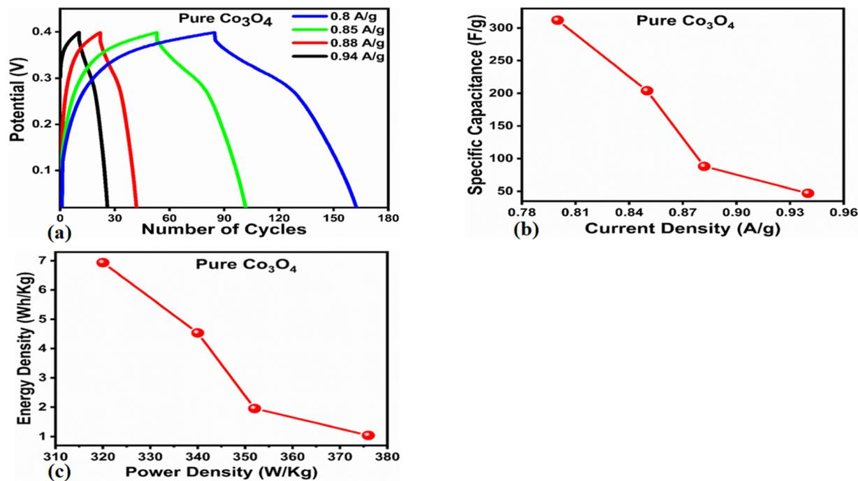
Fig. 9 (a) GCD curves of pure Co<sub>3</sub>O<sub>4</sub> at different current densities. (b) Specific capacitance. (c) Corresponding energy density and power density.
