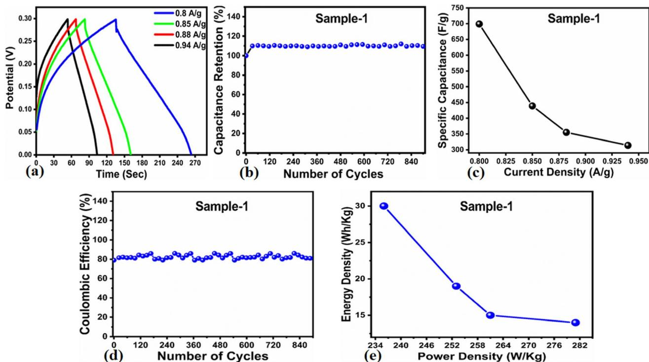
Fig. 10 (a) GCD curves of sample 1 ( $\text{Co}_3\text{O}_4$ ) at different current densities. (b) Percentage retention of specific capacitance. (c) Specific capacitance. (d) Percentage of coulombic efficiency. (e) Energy density and power density.
