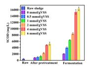
Fig. 4 Variations in SCOD for WAS with different UHP dosages after 1 h pretreatment, Data in fermentation phase were collected at their maximum concentration time.
