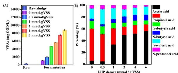
Fig. 5 Variations in (A) VFAs concentration and (B) VFAs composition at the time of maximum VFAs production with different UHP dosages.
