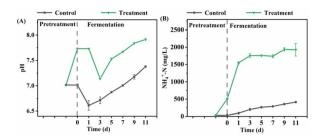
Fig. 8 Variations in (A) pH and (B)  $NH_4^+$ -N after 1 h of pretreatment using 2 mmol UHP per g VSS.
