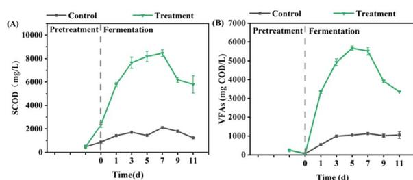
Fig. 1 Performances of pretreatment on (A) WAS hydrolysis and (B) VFAs production after 1 h pretreatment with 2 mmol UHP per g VSS.
