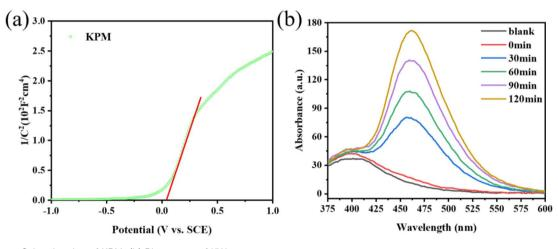
Fig. 11 (a) Mott-Schottky plot of KPM; (b) PL spectra of KW.
