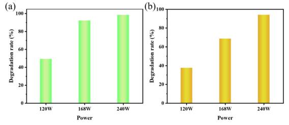
Fig. 9 (a) The effect of ultrasonic power on the sonocatalytic degradation of MO (experimental conditions: sonocatalyst dosage = 50 mg, initial concentration =  $10 \text{ mg L}^{-1}$ , pH = 3); (b) the effect of ultrasonic power on the sonocatalytic degradation of AR88 (experimental conditions: sonocatalyst dosage = 50 mg, initial concentration =  $10 \text{ mg L}^{-1}$ , pH = 7).
