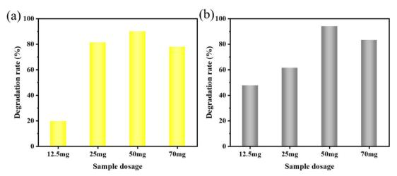
Fig. 6 Effect of different KW sonocatalyst dosages on the sonocatalytic degradation of (a) MO and (b) AR88 (experimental conditions: initial concentration =  $10 \text{ mg L}^{-1}$ , solution volume = 50 mL, ultrasonic power = 240 W, pH = 7).
