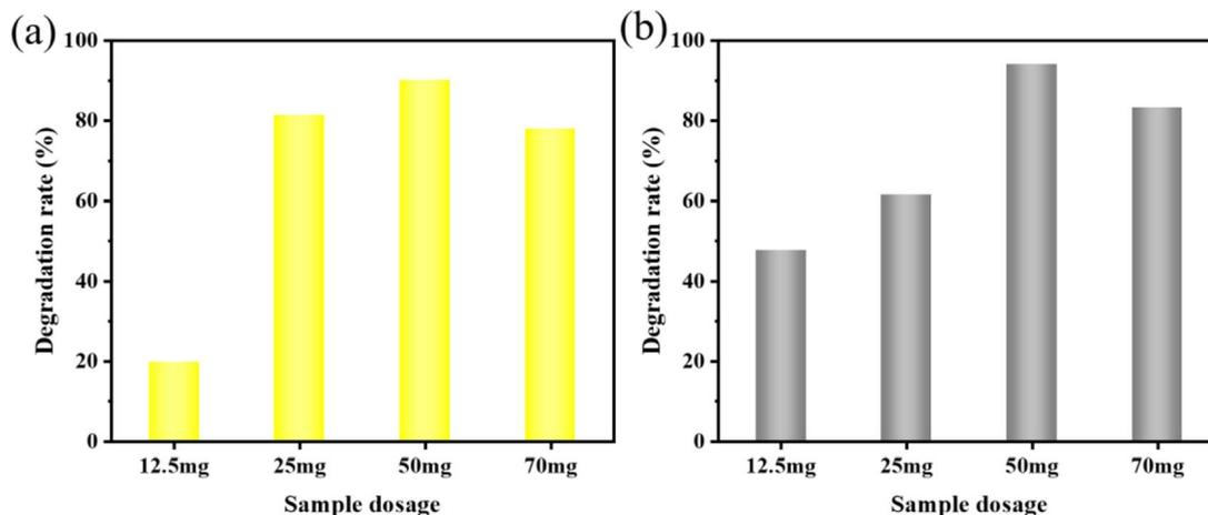
Fig. 6 Effect of different KW sonocatalyst dosages on the sonocatalytic degradation of (a) MO and (b) AR88 (experimental conditions: initial concentration =  $10 \text{ mg L}^{-1}$ , solution volume = 50 mL, ultrasonic power = 240 W, pH = 7).
