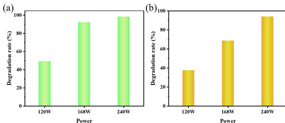
Fig. 9 (a) The effect of ultrasonic power on the sonocatalytic degradation of MO (experimental conditions: sonocatalyst dosage = 50 mg, initial concentration = 10 mg L<sup>-1</sup>, pH = 3); (b) the effect of ultrasonic power on the sonocatalytic degradation of AR88 (experimental conditions: sonocatalyst dosage = 50 mg, initial concentration = 10 mg L<sup>-1</sup>, pH = 7).
