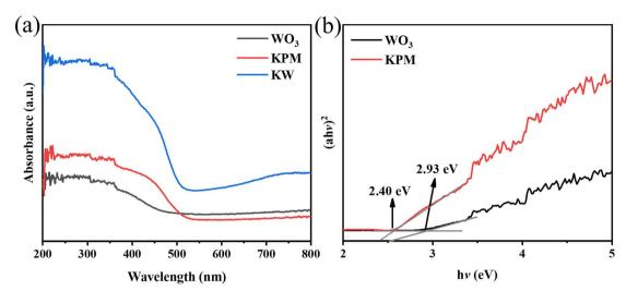
Fig. 4 (a) DRS spectrum of KW; (b) plot of  $(\alpha\hbar\nu)^2 - \hbar\nu$  for WO<sub>3</sub> and KPM samples
