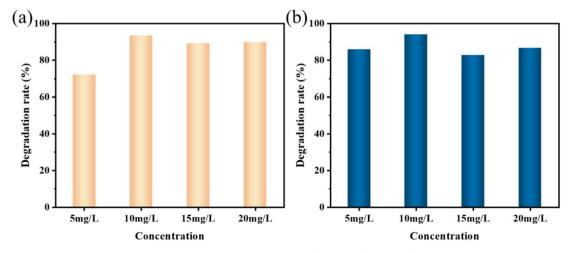
Fig. 7 Sonocatalytic degradation efficiency different initial concentrations of (a) MO and (b) AR88 (experimental conditions: sonocatalyst dosage = 50 mg, solution volume = 50 mL, ultrasonic power = 240 W, pH = 7).
