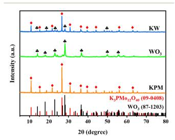
Fig. 1 XRD pattern of WO<sub>3</sub>, KPM, and KW samples.
