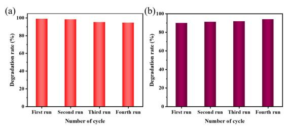
Fig. 10 (a) Results of reusability test for the sonocatalytic degradation of MO (experimental conditions: sonocatalyst dosage = 50 mg, initial MO concentration = 50 mg  $L^{-1}$ , ultrasonic power = 240 W, pH = 3); (b) results of reusability test for the sonocatalytic degradation of AR88 (experimental conditions: sonocatalyst dosage = 50 mg, initial MO concentration = 50 mg  $L^{-1}$ , ultrasonic power = 240 W, pH = 7).
