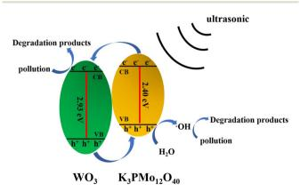
Fig. 12 Possible sonocatalytic mechanism.
