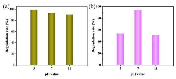
Fig. 8 Effect of different pH values on sonocatalytic degradation of (a) MO and (b) AR88 (experimental conditions: sonocatalyst dosage = 50 mg, solution volume = 50 mL, initial concentration =  $10 \text{ mg L}^{-1}$ , ultrasonic power = 240 W).
