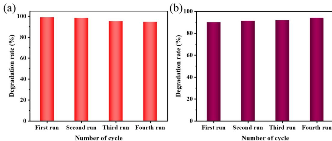
Fig. 10 (a) Results of reusability test for the sonocatalytic degradation of MO (experimental conditions: sonocatalyst dosage = 50 mg, initial MO concentration = 50 mg L<sup>-1</sup>, ultrasonic power = 240 W, pH = 3); (b) results of reusability test for the sonocatalytic degradation of AR88 (experimental conditions: sonocatalyst dosage = 50 mg, initial MO concentration = 50 mg L<sup>-1</sup>, ultrasonic power = 240 W, pH = 7).
