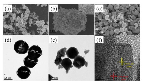
Fig. 2 SEM images of (a) KPM, (b) WO<sub>3</sub>, and (c) KW; TEM images of the (d) KPM, and (e) KW samples; HRTEM image of the (f) KW
