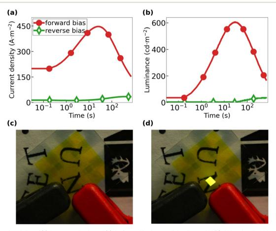
Fig. 3 Temporal evolution of (a) the current density and (b) the forward luminance of the all-organic LEC during electric driving with 40 V, in either forward bias with PEDOT:PSS-2-m being the negative cathode (solid red circles) or in reverse bias with PEDOT:PSS-4-m electrode being the negative cathode (open green diamonds). Photographs of the all-organic LEC (c) in the transparent off-state with no applied voltage and (d) during light emission with 40 V applied in forward bias.
