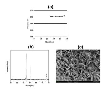
Fig. 10 (a) Chronopotentiometry (CP) for the sample  $CuFeO_x$ -D at a constant J of 100 mA cm<sup>-2</sup> for 50 hours, (b) XRD diffractogram and (c) FESEM image of  $CuFeO_x$ -D after 50 hours stability studies.
