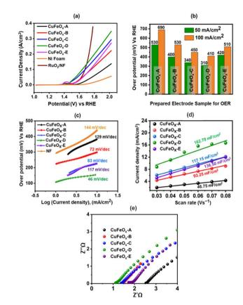
Fig. 7 (a) Polarization curve of prepared electrode samples at 1 M KOH for OER; (b) OP at the J of 100 mA cm $^{-2}$ ; (c) Tafel's slope; (d)  $C_{\rm dl}$  plots of different scan rates vs. J; (e) Nyquist plots of the electrodes.
