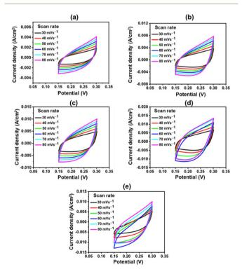
Fig. 9 CV polarization curve at various scan rates; (a) CuFeO<sub>x</sub>-A, (b) CuFeO<sub>x</sub>-B, (c) CuFeO<sub>x</sub>-C, (d) CuFeO<sub>x</sub>-D, and (e) CuFeO<sub>x</sub>-E.
