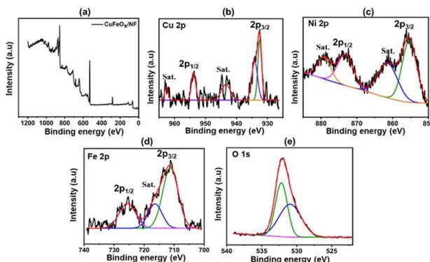
Fig. 6 XPS analysis of CuFeO<sub>x</sub>-D sample; (a) CuFeO<sub>x</sub>-D survey peak, (b) Cu 2p, (c) Ni 2p, (d) Fe 2p, (e) O 1s.
