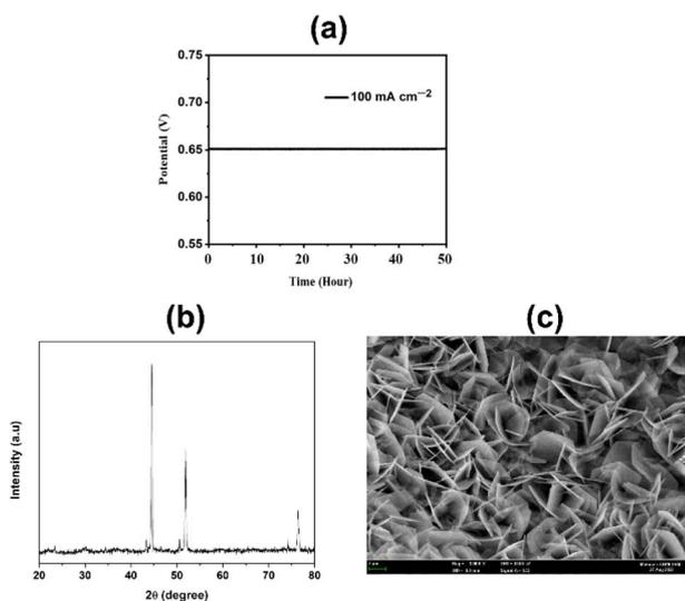
Fig. 10 (a) Chronopotentiometry (CP) for the sample CuFeO<sub>x</sub>-D at a constant  $J$  of 100 mA cm<sup>-2</sup> for 50 hours, (b) XRD diffractogram and (c) FESEM image of CuFeO<sub>x</sub>-D after 50 hours stability studies.
