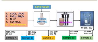
Fig. 1 Schematic diagram of the catalyst preparation process
