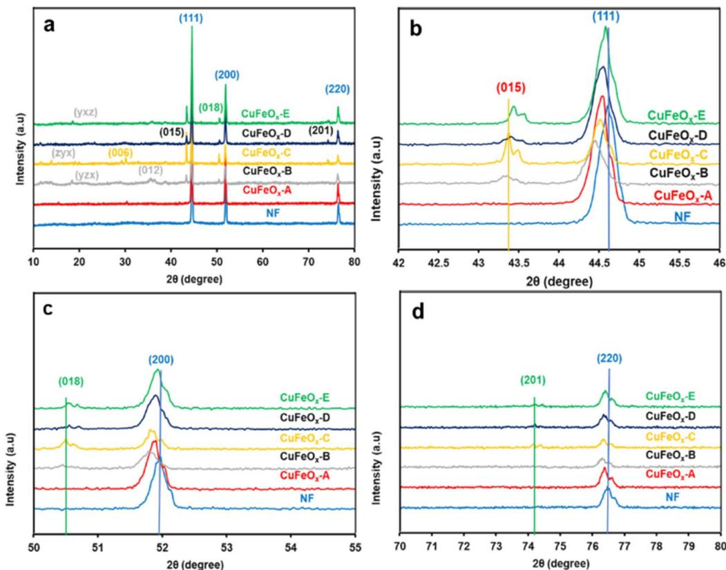
Fig. 2 XRD pattern of the synthesized  $\text{CuFeO}_x$ -based electrode samples and NF; (a) from  $10^\circ$  to  $80^\circ$ , (b) from  $42^\circ$  to  $46^\circ$ , (c) from  $50^\circ$  to  $55^\circ$ , and (d) from  $70^\circ$  to  $80^\circ$ .
