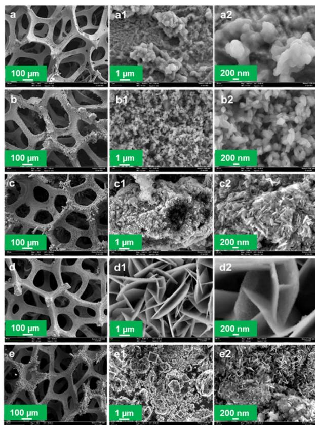
Fig. 3 FESEM images of the prepared electrode samples at different magnifications; (a, a1 and a2) CuFeO<sub>x</sub>-A, (b, b1 and b2) CuFeO<sub>x</sub>-B, (c, c1 and c2) CuFeO<sub>x</sub>-C, (d, d1 and d2) CuFeO<sub>x</sub>-D, and (e, e1 and e2) CuFeO<sub>x</sub>-E.
