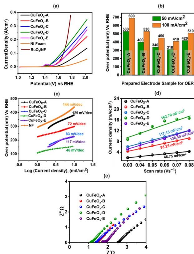
Fig. 7 (a) Polarization curve of prepared electrode samples at 1 M KOH for OER; (b) OP at the *J* of 100 mA cm<sup>-2</sup>; (c) Tafel's slope; (d) *C*<sub>dl</sub> plots of different scan rates vs. *J*; (e) Nyquist plots of the electrodes.
