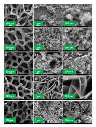
Fig. 3 FESEM images of the prepared electrode samples at different magnifications; (a, a1 and a2)  $CuFeO_x$ -A, (b, b1 and b2)  $CuFeO_x$ -B, (c, c1 and c2)  $CuFeO_x$ -C, (d, d1 and d2)  $CuFeO_x$ -D, and (e, e1 and e2)  $CuFeO_x$ -E.
