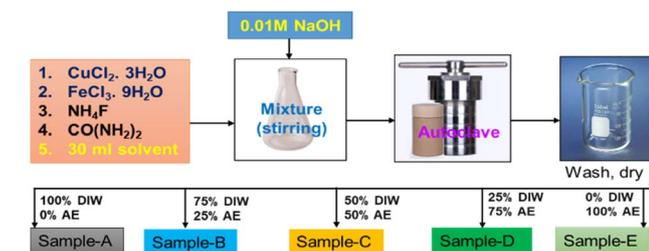
Fig. 1 Schematic diagram of the catalyst preparation process.
