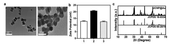
Fig. 2 Preparation and characterization of the UCNPs@Au. (a) TEM analysis of the core-shell UCNPs (NaYF4:Yb, Er@NaYF4) and UCNPs@Au. Scale bar: 100 nm, 50 nm. (b) Zeta potentials of different samples (1: ligand free UCNP; 2: UCNPs@PEI; 3: UCNPs@Au). (c) XRD spectra of UCNPs@Au, standard card of β-NaYF<sub>4</sub> (JCPDS no. 16-0334), and Au (JCPDS no. 65-2870)
