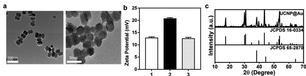
Fig. 2 Preparation and characterization of the UCNPs@Au. (a) TEM analysis of the core-shell UCNPs (NaYF<sub>4</sub>:Yb, Er@NaYF<sub>4</sub>) and UCNPs@Au. Scale bar: 100 nm, 50 nm. (b) Zeta potentials of different samples (1: ligand free UCNP; 2: UCNPs@PEI; 3: UCNPs@Au). (c) XRD spectra of UCNPs@Au, standard card of β-NaYF<sub>4</sub> (JCPDS no. 16-0334), and Au (JCPDS no. 65-2870).
