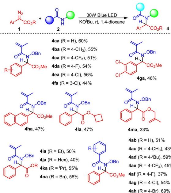
Scheme 3 Substrate scope with 1,4-dioxane as the solvent. Reaction conditions: **1** (0.2 mmol), **2** (0.3 mmol), KO<sup>t</sup>Bu (0.24 mmol), 1,4-dioxane (2 mL), r.t., 30W blue LEDs ( $\lambda \approx 440-450$  nm), 14 h. Isolated yield.
