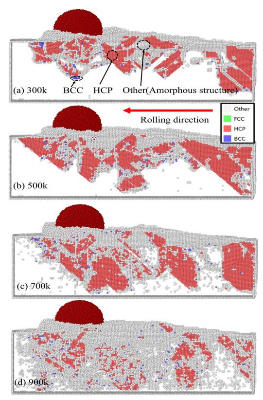
Fig. 9 Schematic diagram of defect atom distribution.
