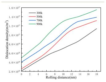
Fig. 7 Dislocation density at different rolling temperatures.
