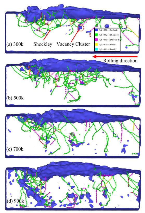
Fig. 8 Dislocation type distribution diagram.
