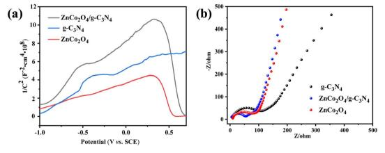
Fig. 9 (a) Mott-Schottky and (b) electrochemical impedance spectroscopy of samples.
