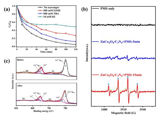
Fig. 8 (a) The quenching experiments using EtOH, TBA, and KI. (b) DMPO- $^{\bullet}$ OH and DMPO-SO<sub>4</sub> $^{\bullet}$  adduct in ESR spectra under different conditions. (c) Co 2p XPS spectrum of ZnCo<sub>2</sub>O<sub>4</sub>/g-C<sub>3</sub>N<sub>4</sub> catalyst before and after reaction.
