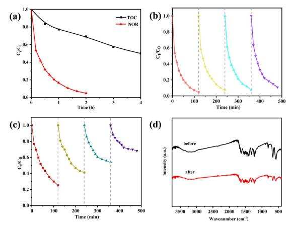
Fig. 7 (a) TOC removal and NOR degradation during the reaction; recycle experiments of NOR removal for (b)  $ZnCo_2O_4/g-C_3N_4$  and (c)  $ZnCo_2O_4$  catalyst; (d) FTIR spectra of fresh and used  $ZnCo_2O_4/g-C_3N_4$  catalyst.
