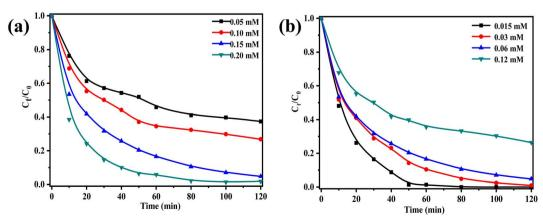
Fig. 5 Comparison the performance of ZnCo<sub>2</sub>O<sub>4</sub>/q-C<sub>3</sub>N<sub>4</sub> under different conditions: (a) PMS dosage, (b) initial NOR concentration.
