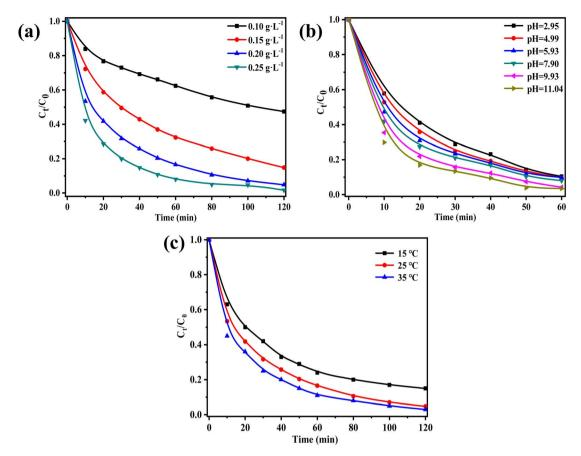
Fig. 6 Comparison the performance of  $ZnCo_2O_4/g-C_3N_4$  under different conditions: (a) catalyst dosage, (b) initial pH value, (c) temperature.
