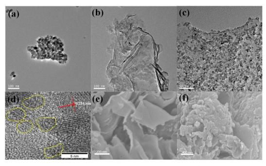
Fig. 1 TEM images of (a)  $ZnCo_2O_4$ , (b)  $g-C_3N_4$ , (c)  $ZnCo_2O_4/g-C_3N_4$ ; (d) HRTEM image of  $ZnCo_2O_4/g-C_3N_4$ ; and SEM images of (e)  $g-C_3N_4$  and (f)  $ZnCo_2O_4/g-C_3N_4$ .
