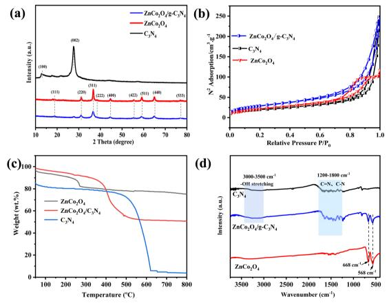
Fig. 2 (a) XRD patterns. (b)  $N_2$  adsorption-desorption isotherms. (c) TGA, and (d) FTIR spectra of  $ZnCo_2O_4$ ,  $g-C_3N_4$  and  $ZnCo_2O_4/g-C_3N_4$ .
