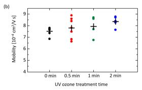
Fig. 4 Electrical characteristics of spiro-OMeTAD films as a function of UV ozone treatment time. (a) Conductivity measured for /ITO/spiro-OMeTAD/Au device. (b) Hole mobility measured for ITO/PEDOT:PSS/spiro-OMeTAD/Au device.
