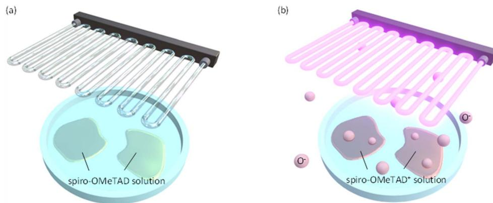
Fig. 1 Schematic depiction of UV ozone treatment for spiro-OMeTAD in solution. (a) Before and (b) after the treatments. The  $O^-$  ions generated by a UV ozone treatment promote oxidation of spiro-OMeTAD molecule. After oxidation, solution is used for spin-coating.
