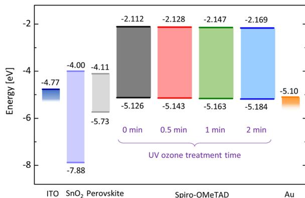
Fig. 3 HOMO and LUMO levels of UV ozone treated spiro-OMeTAD films and energy diagram in solar cell device. Energies for spiro-OMeTAD and perovskite were evaluated from absorption and PYS measurements.
