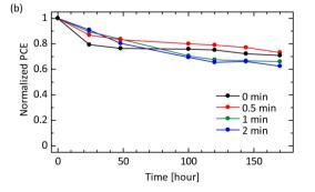
Fig. 5 Photovoltaic characterization of perovskite solar cell with UV ozone treated spiro-OMeTAD HTL. (a) Normalized PCE of solar cell samples at various UV ozone treatment times. The data are normalized by the averaged PCE of devices without the treatment. (b) Evolution of the normalized PCE of devices left in an atmospheric environment.
