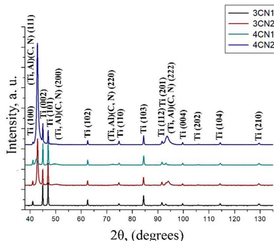
**Fig. 5** X-ray diffraction patterns of the TiAlCuCN coating. Substrate – Titanium Grade 2.
