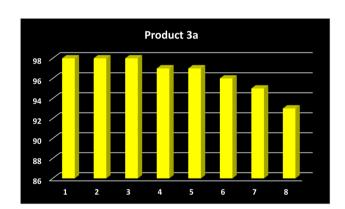
Fig. 9 Reusability of MNP-[Dop-OH]-CuBr $_2$  nanocatalysts in the preparation of product  ${\bf 3a}$ .
