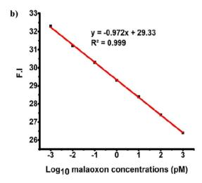
Fig. 6 The effect of malaoxon in AgNPs aggregation on GO (a) fluorescence spectra of AChE-ATCh-Ag-GO with varied concentrations of malaoxon (0.001 pM to 1000 pM) (b) straight line calibration plot for log<sub>10</sub> malaoxon concentrations and FI.
