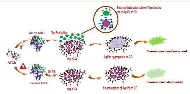
Fig. 3 Schematic illustration for the detection principle of malaoxon using AChE-ATCh-Ag-GO.
