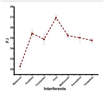
Fig. 7 Evaluation of the anti-interference ability of the AChE-ATCh-Ag-GO system.
