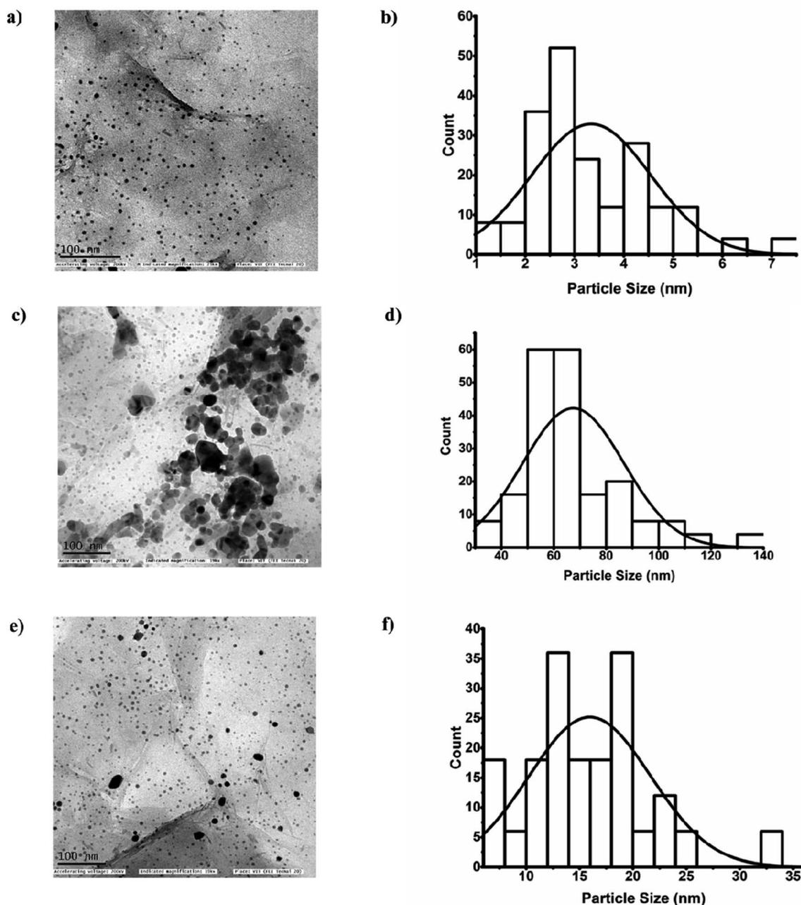
Fig. 5 HR-TEM images of (a) Ag-GO and (b) particle size histogram of AgNPs on GO (c) AChE-ATCh-Ag-GO (d) particle size histogram of AgNPs on GO with AChE, and ATCh (e) AChE-ATCh-Ag-GO with malaoxon (1000 pM) (f) particle size histogram of AgNPs on GO with AChE, ATCh and malaoxon (1000 pM).
