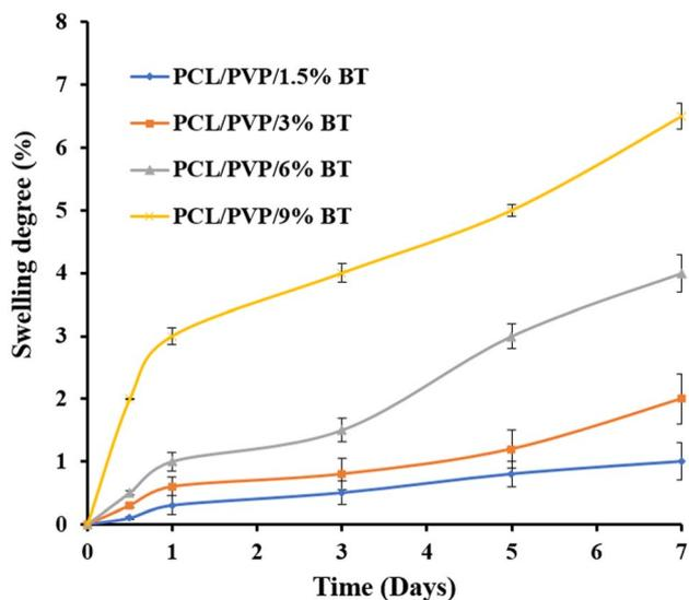
Fig. 4 Swelling ratio of different BT-loaded nanofibrous scaffolds.
