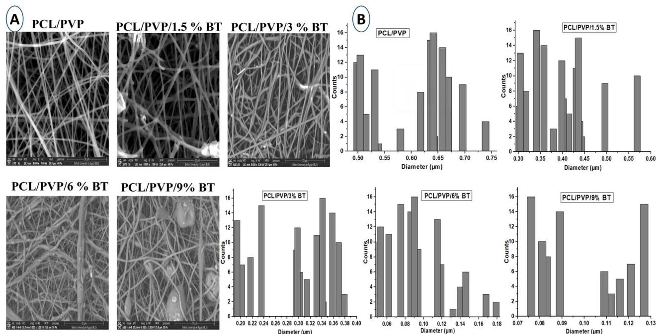
Fig. 3 (A) SEM images of PCL/PVP, PCL/PVP/1.5% BT, PCL/PVP/3% BT, PCL/PVP/6% BT, PCL/PVP/9% BT, (original magnification 8000 $\times$ ; scale 10  $\mu$ m), and (B) the average diameter of nanofibers for loaded and unloaded scaffolds.
