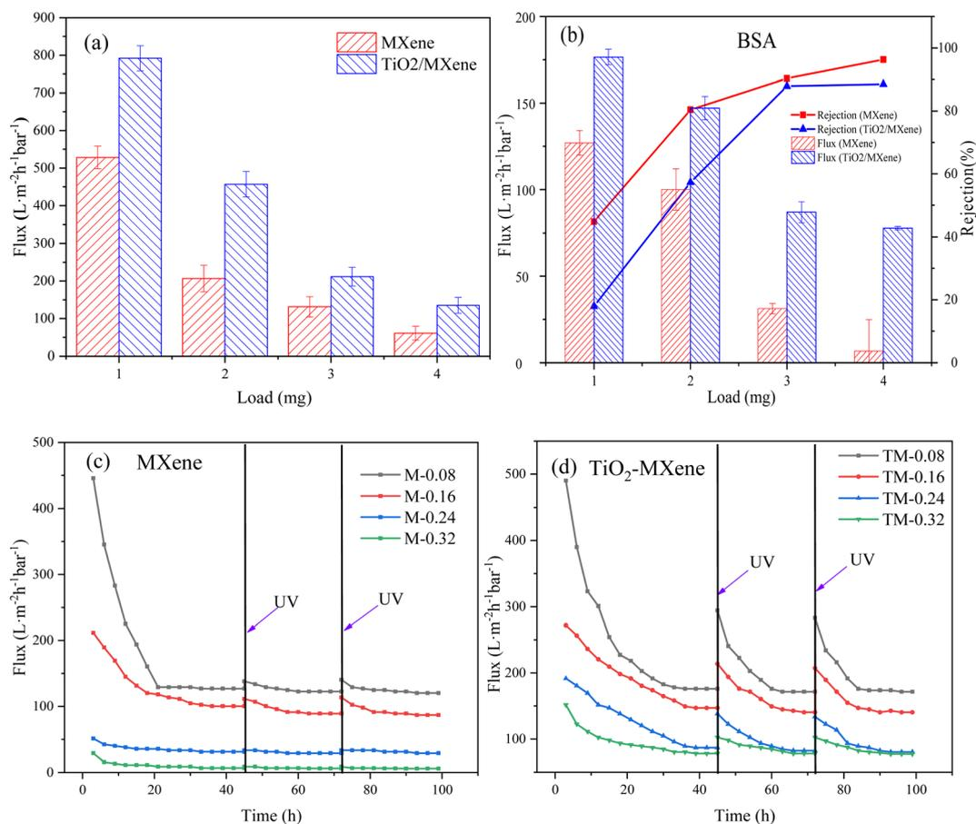
Fig. 4 Membranes (a) pure water flux and (b) BSA retention and stabilization flux, UV self-cleaning ability of (c) MXene and (d) TiO<sub>2</sub>/MXene membranes under BSA contamination.
