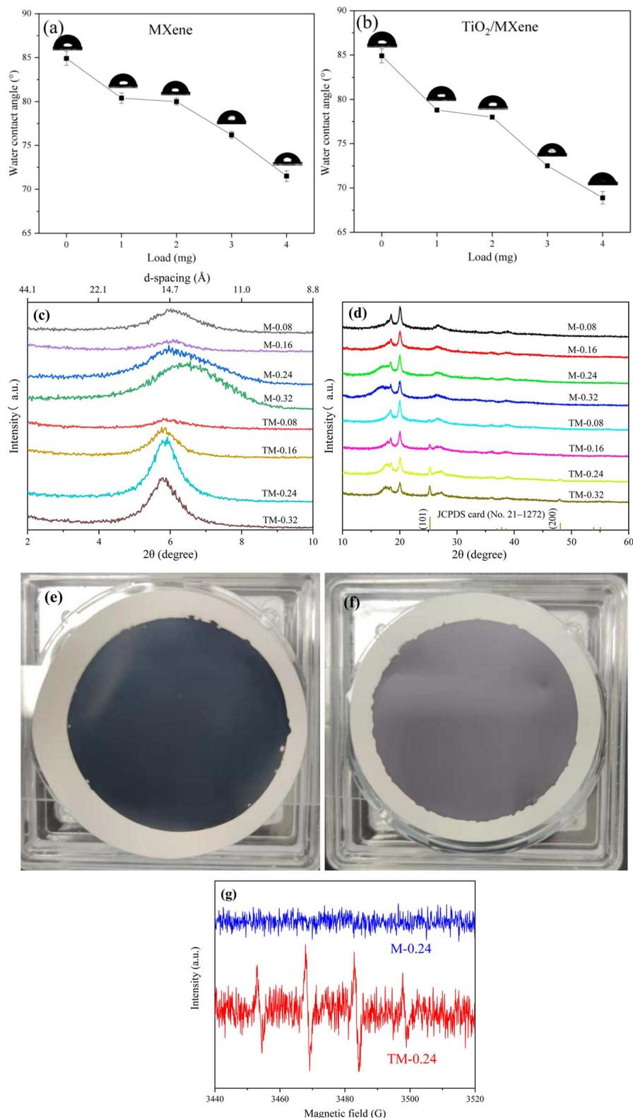
Fig. 3 Water contact angles of (a) MXene and (b) TiO<sub>2</sub>/MXene membranes, (c) XRD small-angle diffraction image, (d) XRD image of the eight membranes and pictures of (e) M-0.24, (f) TM-0.24. (g) EPR curves of hydroxyl radicals.
