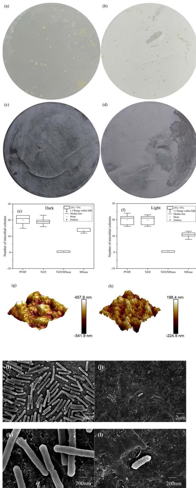
Fig. 6 Microbial growth of (a) PVDF membrane, (b) nano- $\text{TiO}_2$  loaded membrane, (c) M-0.24, (d) TM-0.24, and (e) bacterial growth numbers of the membrane under (e) dark, (f) light conditions, AFM images of (g) M-0.24 and (h) TM-0.24, SEM low magnification images of the *E. coli* colonies grown on (i) M-0.24 and (j) TM-0.24, high magnification images of *E. coli* grown on (k) M-0.24 and (l) TM-0.24.
