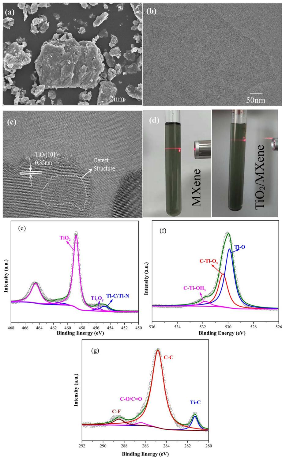
Fig. 1 (a) SEM of MAX material; (b) TEM of monolayer MXene; (c) high resolution TEM of monolayer  $\text{TiO}_2/\text{MXene}$ ; (d) Tyndall effect of dilute solution at  $0.02 \text{ mg mL}^{-1}$ ; XPS of (e) Ti 2p, (f) O 1s and (g) C 1s of  $\text{TiO}_2/\text{MXene}$ .
