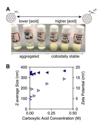
Fig. 6 (A) COF-300 colloids that have been fully purified *via* centrifugation are colloidally stable in acetonitrile only in the presence of added benzoic acid. (B) Z-average size (nm) (represented as filled triangles) and zeta potential (mV) (represented as unfilled triangles) of COF-300 colloids purified *via* centrifugation and resuspended in benzonitrile as a function of carboxylic acid concentration.
