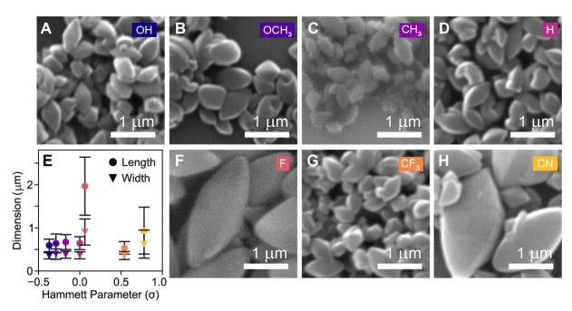
Fig. 3 (A–D, F–H) SEM of COF-300 colloids synthesized at 90 °C for 48 hours made from different benzoic acids. (E) Average colloid length and width distribution data plotted vs. Hammett parameter.
