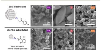
Fig. 7 SEM images comparing COF-300 particle sizes as synthesized with (A–C) para-substituted benzoic acids ( $X = CH_3$ , F,  $CF_3$ ) vs. particles synthesized with (D–F) diortho-substituted benzoic acids ( $X = CH_3$ , F,  $CF_3$ ).
