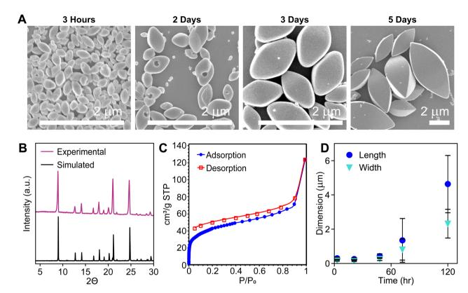
Fig. 1 (A) SEM images of colloidal COF-300 (X = H) particle growth at 90 °C, (B) PXRD: experimental data (top) and simulated hydrated COF-300 pattern (bottom),  $^{1}$  (C) N<sub>2</sub> adsorption isotherm, and (D) dimensions as determined *via* SEM measurements.
