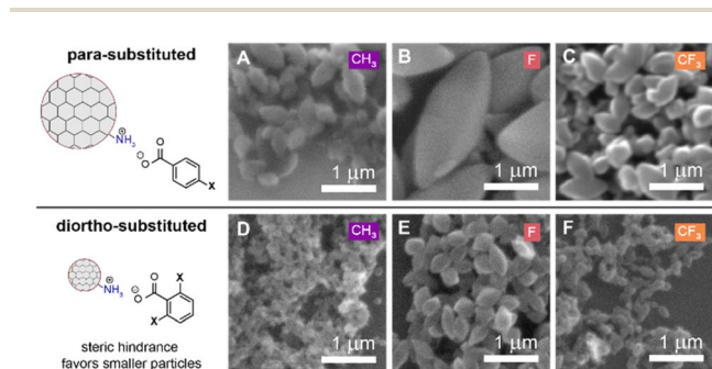
Fig. 7 SEM images comparing COF-300 particle sizes as synthesized with (A–C) para -substituted benzoic acids ( X = \text{CH}_3, \text{F}, \text{CF}_3 ) vs. particles synthesized with (D–F) diortho-substituted benzoic acids ( X = \text{CH}_3, \text{F}, \text{CF}_3 ).
