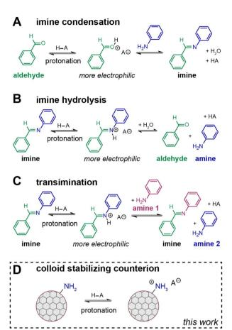
Scheme 3 Acid plays multiple roles in imine-linked COF colloid synthesis including (A) acid-catalyzed imine condensation, (B) acid-catalyzed imine hydrolysis, (C) acid-catalyzed transimination, and (D) a colloid stabilizing counterion via formation of an acid-base adduct.
