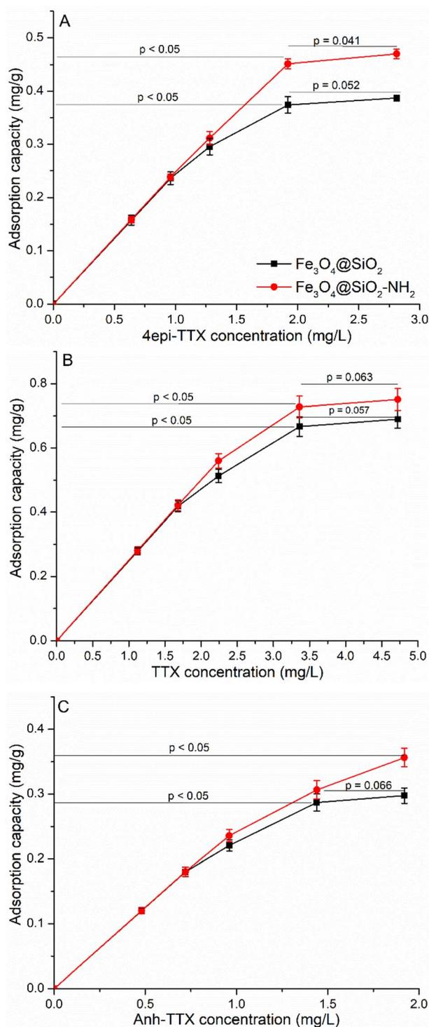
Fig. 7 Adsorption capacity of Fe<sub>3</sub>O<sub>4</sub>@SiO<sub>2</sub> and Fe<sub>3</sub>O<sub>4</sub>@SiO<sub>2</sub>-NH<sub>2</sub> for 4epi-TTX (A), TTX (B) and Anh-TTX (C) under different initial concentrations of 4epi-TTX, TTX, and Anh-TTX. Adsorption conditions: temperature, 25 °C; pH, 2.0; stirring rate, 150 rpm; adsorbent dosage, 4 g L<sup>-1</sup>; contact time, 50 min.
