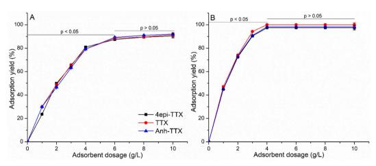
Fig. 6 Adsorption yield of  $Fe_3O_4$ @Si $O_2$  (A) and  $Fe_3O_4$ @Si $O_2$ -NH<sub>2</sub> (B) for 4epi-TTX, TTX and Anh-TTX under different  $Fe_3O_4$ @Si $O_2$  and  $Fe_3$ -O<sub>4</sub>@Si $O_2$ -NH<sub>2</sub> dosages. Adsorption conditions: temperature, 25 °C; pH, 2.0; stirring rate, 150 rpm; initial adsorbate concentrations, 1.28 mg L<sup>-1</sup> 4epi-TTX, 2.24 mg L<sup>-1</sup> TTX and 0.96 mg L<sup>-1</sup> Anh-TTX; contact time, 50 min.
