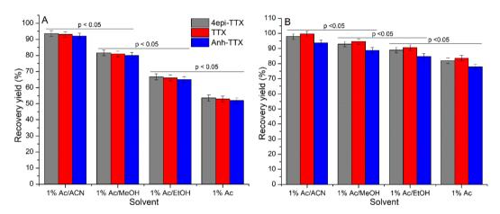
Fig. 9 Recovery yield of 4epi-TTX, TTX, and Anh-TTX from  $Fe_3O_4@SiO_2$ -TTX (A) and  $Fe_3O_4@SiO_2$ -NH<sub>2</sub>-TTX (B) using different solvents. Adsorption conditions: temperature, 40 °C; pH, 2.0; stirring rate, 150 rpm; adsorbent dosage, 4 g L<sup>-1</sup>; initial adsorbate concentrations, 1.92 mg L<sup>-1</sup> 4epi-TTX, 3.36 mg L<sup>-1</sup> TTX, and 1.44 mg L<sup>-1</sup> Anh-TTX; contact time, 50 min. Desorption conditions: temperature: 50 °C, extraction time 30 min.
