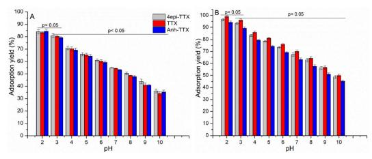
Fig. 5 Adsorption yield of  $Fe_3O_4$ @SiO<sub>2</sub> (A) and  $Fe_3O_4$ @SiO<sub>2</sub>  $-NH_2$  (B) for 4epi-TTX, TTX, and Anh-TTX under different pH. Adsorption conditions: temperature, 25 °C; stirring rate, 150 rpm; adsorbent dosage, 4 g L<sup>-1</sup>; initial adsorbate concentrations, 1.28 mg L<sup>-1</sup> 4epi-TTX, 2.24 mg L<sup>-1</sup> TTX and 0.96 mg L<sup>-1</sup> Anh-TTX; contact time, 50 min.
