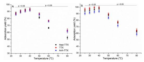
Fig. 8 Adsorption yield of  $Fe_3O_4$ @Si $O_2$  (A) and  $Fe_3O_4$ @Si $O_2$ -NH $_2$  (B) for 4epi-TTX, TTX, and Anh-TTX at different temperatures. Adsorption conditions: pH, 2.0; stirring rate, 150 rpm; adsorbent dosage, 4 g L $^{-1}$ ; initial adsorbate concentrations, 1.92 mg L $^{-1}$  4epi-TTX, 3.36 mg L $^{-1}$  TTX, and 1.44 mg L $^{-1}$  Anh-TTX; contact time, 50 min.
