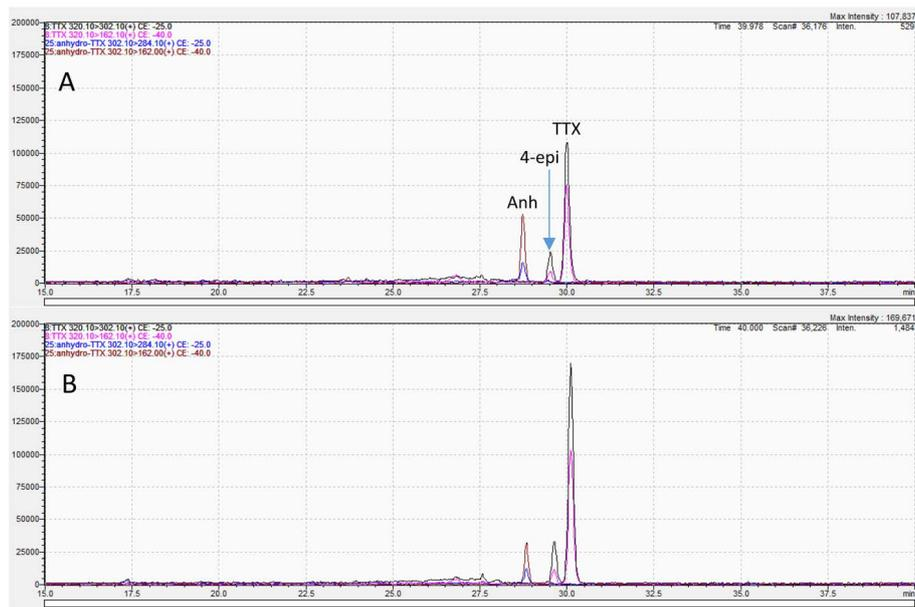
Fig. 10 HPLC spectra of 4epi-TTX, TTX, and Anh-TTX recovered from  $\text{Fe}_3\text{O}_4@SiO_2$ -TTX (A) and  $\text{Fe}_3\text{O}_4@SiO_2$ -NH<sub>2</sub>-TTX (B) using 1% AA/ACN solvent.
