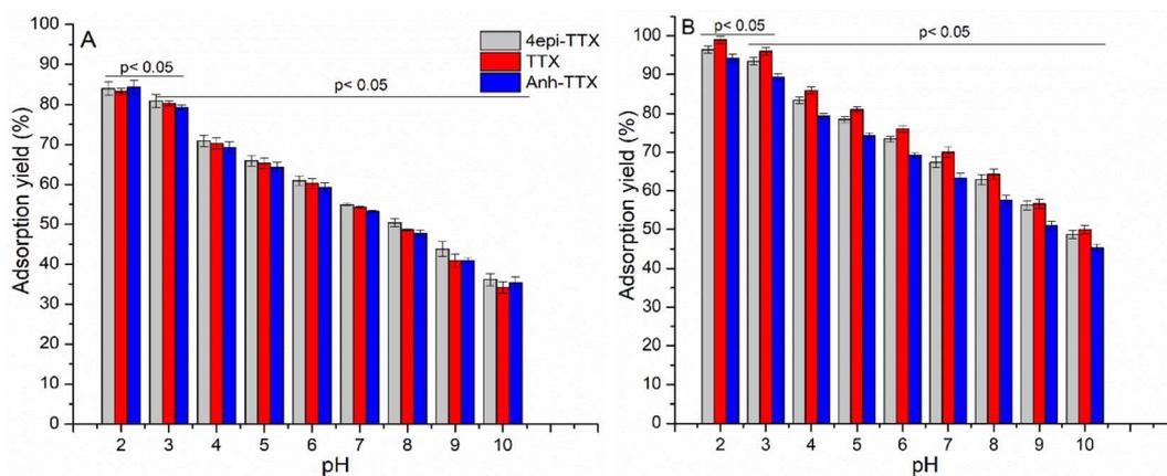
Fig. 5 Adsorption yield of Fe<sub>3</sub>O<sub>4</sub>@SiO<sub>2</sub> (A) and Fe<sub>3</sub>O<sub>4</sub>@SiO<sub>2</sub>-NH<sub>2</sub> (B) for 4epi-TTX, TTX, and Anh-TTX under different pH. Adsorption conditions: temperature, 25 °C; stirring rate, 150 rpm; adsorbent dosage, 4 g L<sup>-1</sup>; initial adsorbate concentrations, 1.28 mg L<sup>-1</sup> 4epi-TTX, 2.24 mg L<sup>-1</sup> TTX and 0.96 mg L<sup>-1</sup> Anh-TTX; contact time, 50 min.
