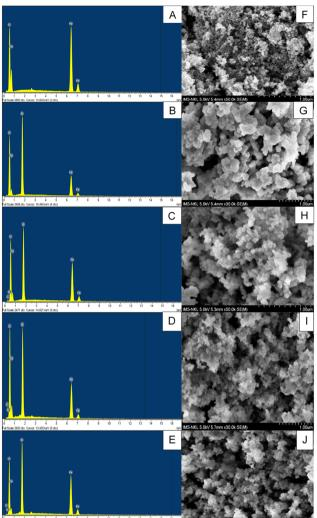
Fig. 2 EDS spectra of Fe $_3$ O $_4$  (A), Fe $_3$ O $_4$ @SiO $_2$  (B), Fe $_3$ O $_4$ @SiO $_2$ -NH $_2$  (C), Fe $_3$ O $_4$ @SiO $_2$ -TTX (D), Fe $_3$ O $_4$ @SiO $_2$ -NH $_2$ -TTX (E) and SEM image of Fe $_3$ O $_4$  (F), Fe $_3$ O $_4$ @SiO $_2$  (G), Fe $_3$ O $_4$ @SiO $_2$ -NH $_2$  (H), Fe $_3$ O $_4$ @SiO $_2$ -TTX (J), Fe $_3$ O $_4$ @SiO $_2$ -NH $_2$ -TTX (J).
