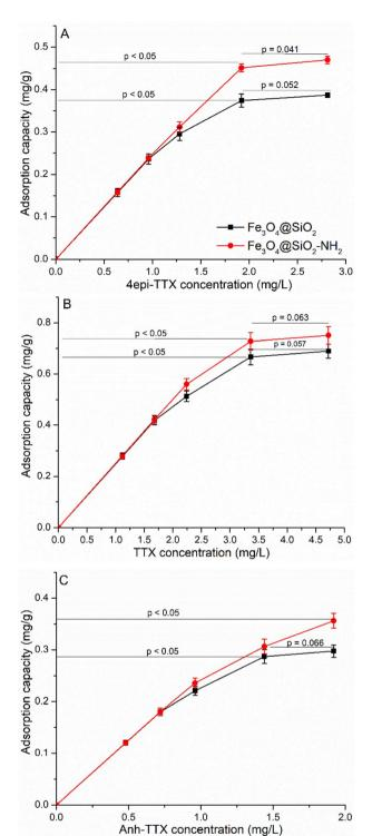
Fig. 7 Adsorption capacity of  $Fe_3O_4$ @Si $O_2$  and  $Fe_3O_4$ @Si $O_2$ -NH $_2$  for 4epi-TTX (A), TTX (B) and Anh-TTX (C) under different initial concentrations of 4epi-TTX, TTX, and Anh-TTX. Adsorption conditions: temperature, 25 °C; pH, 2.0; stirring rate, 150 rpm; adsorbent dosage, 4 g L $^{-1}$ ; contact time, 50 min.
