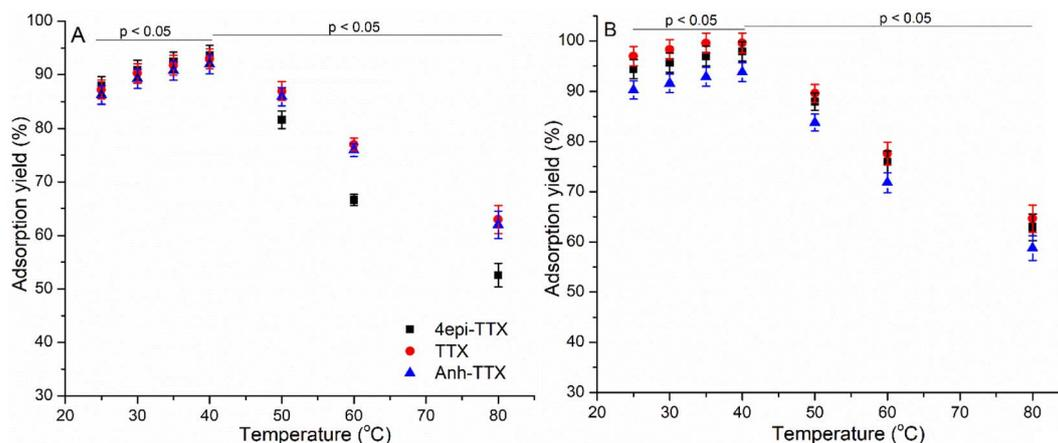
Fig. 8 Adsorption yield of  $\text{Fe}_3\text{O}_4@\text{SiO}_2$  (A) and  $\text{Fe}_3\text{O}_4@\text{SiO}_2\text{-NH}_2$  (B) for 4epi-TTX, TTX, and Anh-TTX at different temperatures. Adsorption conditions: pH, 2.0; stirring rate, 150 rpm; adsorbent dosage,  $4 \text{ g L}^{-1}$ ; initial adsorbate concentrations,  $1.92 \text{ mg L}^{-1}$  4epi-TTX,  $3.36 \text{ mg L}^{-1}$  TTX, and  $1.44 \text{ mg L}^{-1}$  Anh-TTX; contact time, 50 min.
