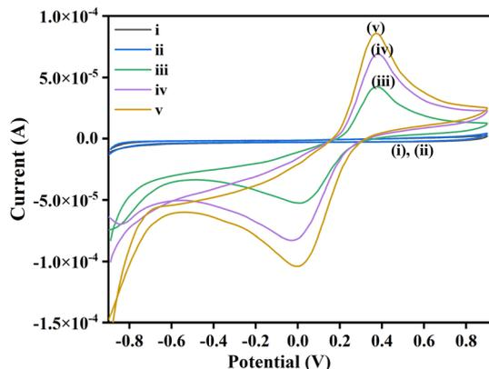
Fig. 5 Cyclic voltammograms in the standard electrolyte: (i) **1a**, (ii) **2a**, (iii)  $I_2 + 2a$ , (iv)  $I_2 + 1a$ , (v)  $I_2$ .
