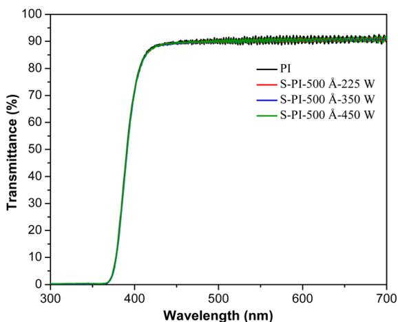
Fig. 7 UV-vis spectra of original PI and remaining PI substrates after etching AR layer from S-PI-500 Å- $\gamma$  films. Etching the AR layer.
