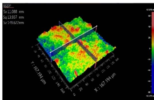
Fig. 3 WLI image of PI substrate.
