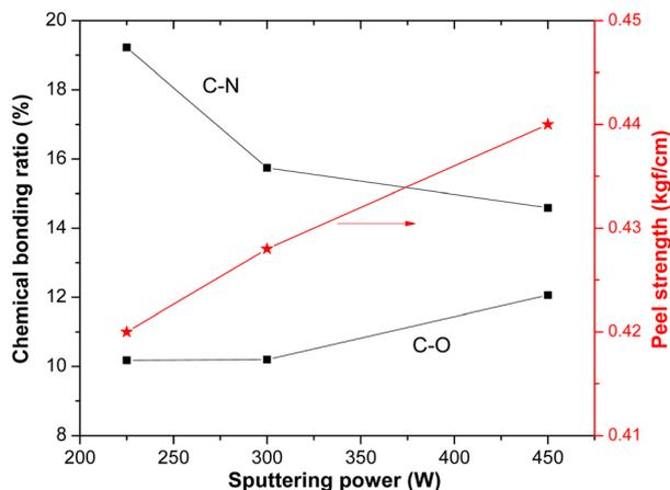
Fig. 6 Effects of sputtering power ( $\gamma$ ) on the chemical bonding ratio and peel strength of S-PI-500 Å- $\gamma$  films.
