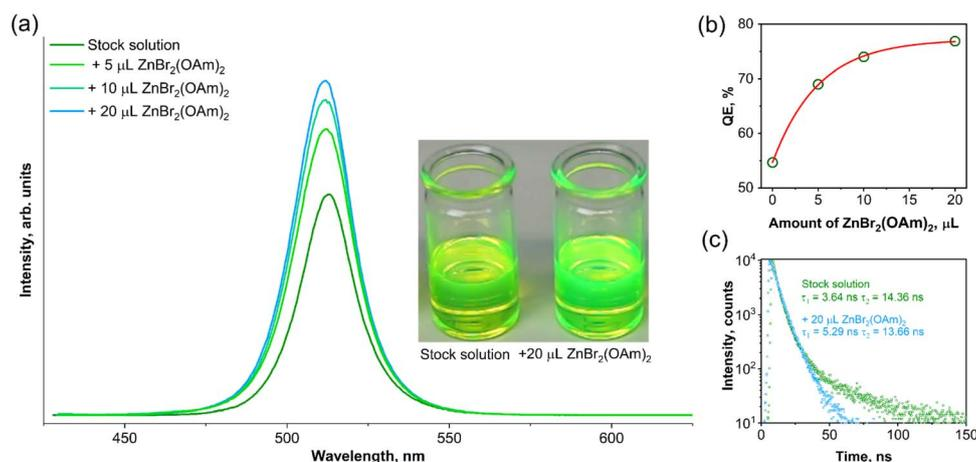
Fig. 3 Evolution of emission spectra ( $\lambda_{\text{ex}} = 365 \text{ nm}$ ) intensity (a) and QEs (b) of CsPbBr<sub>3</sub> QDs in toluene as a function of the added amount of ZnBr<sub>2</sub> complex; PL decay curves of stock CsPbBr<sub>3</sub> QDs solution and solution treated with 20  $\mu\text{L}$  of ZnBr<sub>2</sub> complex (c). The visual color difference of stock and modified CsPbBr<sub>3</sub> QDs solutions at daylight (insert in (a)).
