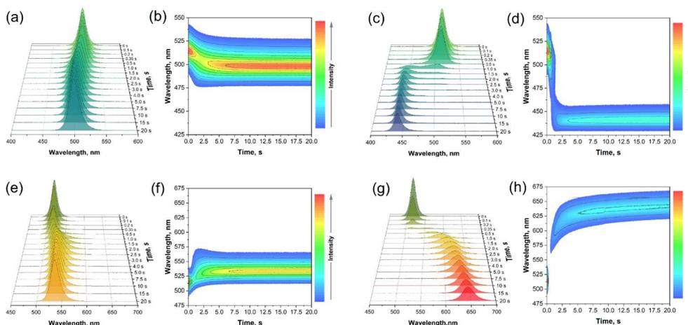
**Fig. 4** Evolution of emission spectra as a function of time and the contour plot of CsPbBr<sub>3</sub> QDs during post-synthesis treatment with 50  $\mu$ L ZnCl<sub>2</sub>(OAm)<sub>2</sub> (a, b); 500  $\mu$ L ZnCl<sub>2</sub>(OAm)<sub>2</sub> (c, d); 50  $\mu$ L ZnI<sub>2</sub>(OAm)<sub>2</sub> (e, f) and 500  $\mu$ L ZnI<sub>2</sub>(OAm)<sub>2</sub> (g, h) complex solutions.
