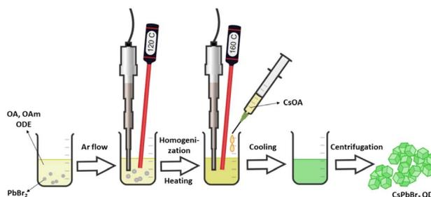
Fig. 1 The synthesis scheme of all-inorganic perovskite QDs.
