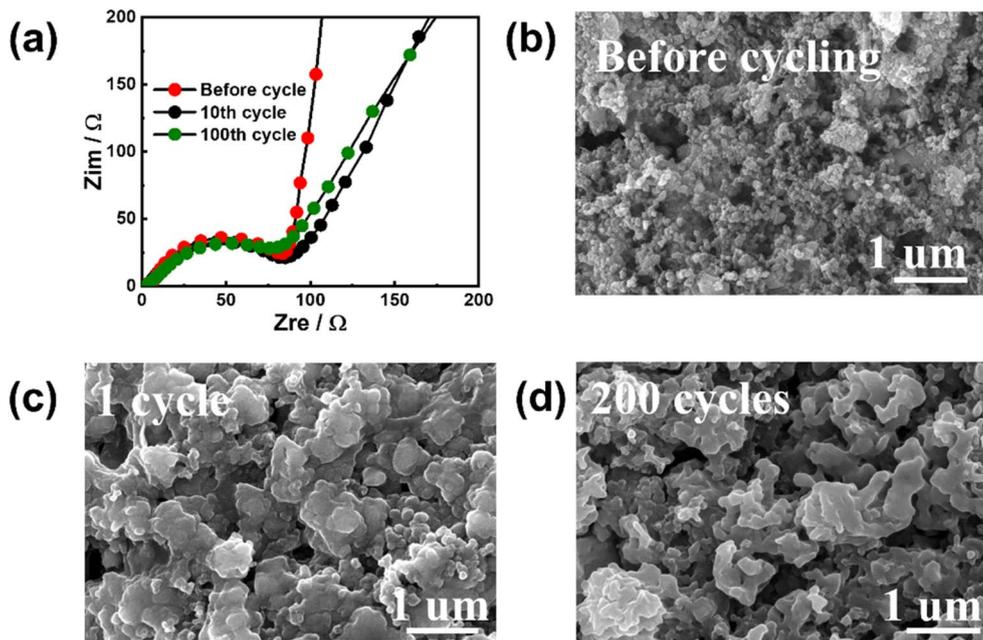
Fig. 5 (a) EIS variations of Sb–PMA–300 electrode during cycling; Morphology of Sb–PMA–300 electrodes (b) before cycling, after (c) 1 cycle and (d) 200 cycles.
