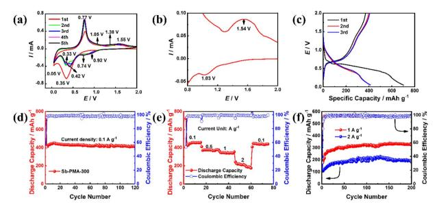
Fig. 4 Electrochemical properties of Sb-PMA-300: (a) the first five CV curves at 0.2 mV s<sup>-1</sup>, (b) partial amplification of the first CV curve in (a), (c) the first three charge and discharge profiles at 0.1 A g<sup>-1</sup>, (d) cycle performance at 0.1 A g<sup>-1</sup>, (e) rate capability, and (f) cycle performance at 1 A g<sup>-1</sup> and 2 A g<sup>-1</sup>.
