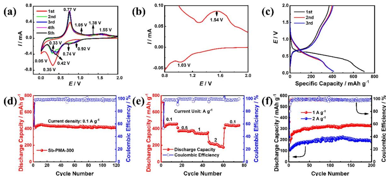
Fig. 4 Electrochemical properties of Sb-PMA-300: (a) the first five CV curves at  $0.2 \text{ mV s}^{-1}$ , (b) partial amplification of the first CV curve in (a), (c) the first three charge and discharge profiles at  $0.1 \text{ A g}^{-1}$ , (d) cycle performance at  $0.1 \text{ A g}^{-1}$ , (e) rate capability, and (f) cycle performance at  $1 \text{ A g}^{-1}$  and  $2 \text{ A g}^{-1}$ .
