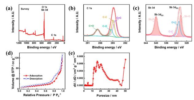
Fig. 3 (a) XPS survey, (b) C 1s HRXPS, (c) O 1s and Sb 3d HRXPS, (d)  $N_2$  adsorption and desorption isotherms and (e) pore size distribution curve of Sb-PMA-300.
