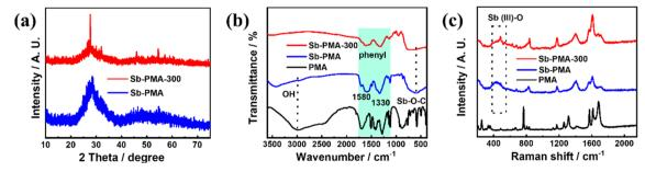
Fig. 2 (a) XRD patterns, (b) FTIR spectra and (c) Raman spectra of Sb-PMA-300.
