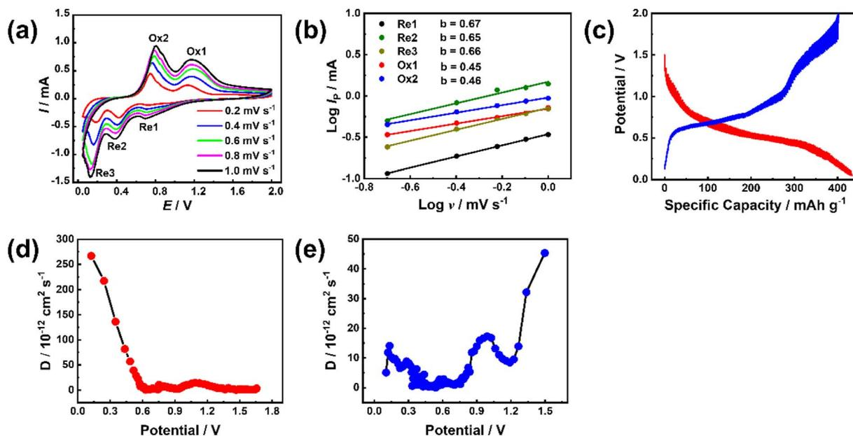
Fig. 6 (a) CV curves and (b) linear relationship between  $\log(I_p)$  versus  $\log(v)$  of Sb-MOF-300 at 0.2–1.0  $mV s^{-1}$ ; (c) GITT curves, variation of  $D$  value of Sb-MOF-300 during (d) discharging and (e) charging.
