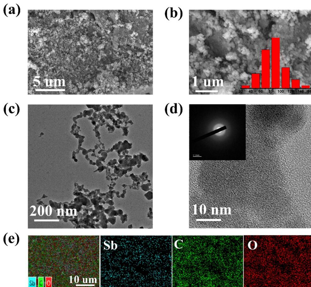
Fig. 1 (a and b) SEM images, (c and d) TEM image and HRTEM image with SAED pattern, (e) element distribution maps of Sb–PMA-300.
