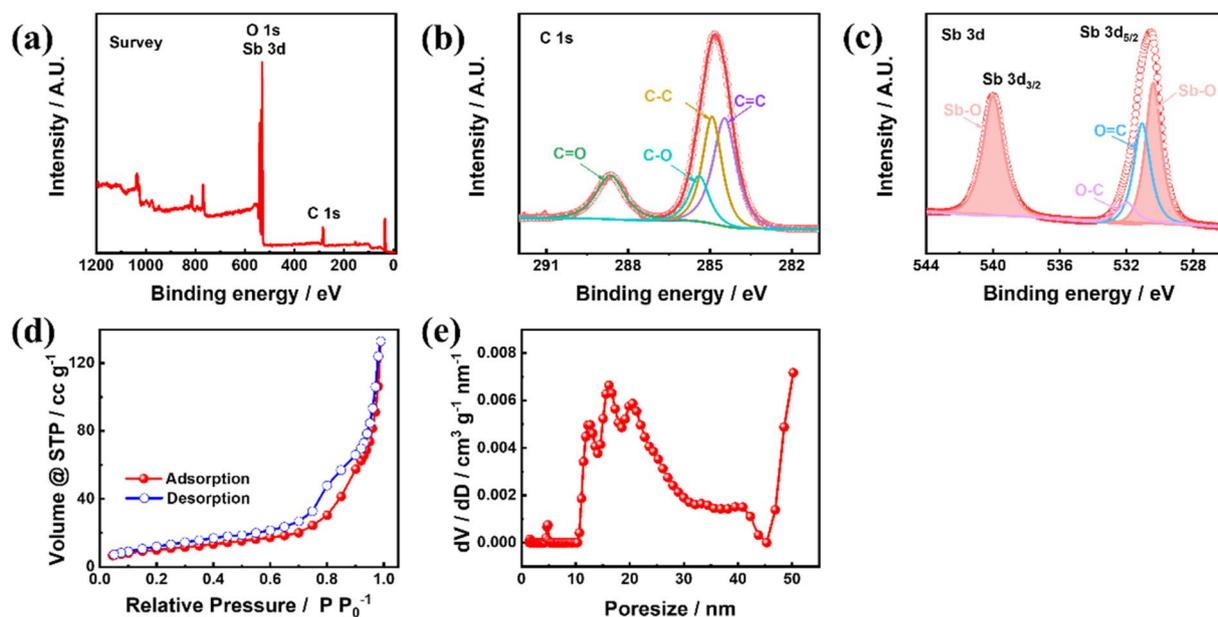
Fig. 3 (a) XPS survey, (b) C 1s HRXPS, (c) O 1s and Sb 3d HRXPS, (d)  $\text{N}_2$  adsorption and desorption isotherms and (e) pore size distribution curve of Sb–PMA-300.
