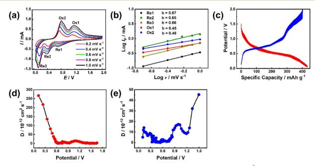
Fig. 6 (a) CV curves and (b) linear relationship between  $log(I_p)$  versus log(v) of Sb-MOF-300 at 0.2–1.0 mV s<sup>-1</sup>; (c) GITT curves, variation of D value of Sb-MOF-300 during (d) discharging and (e) charging.
