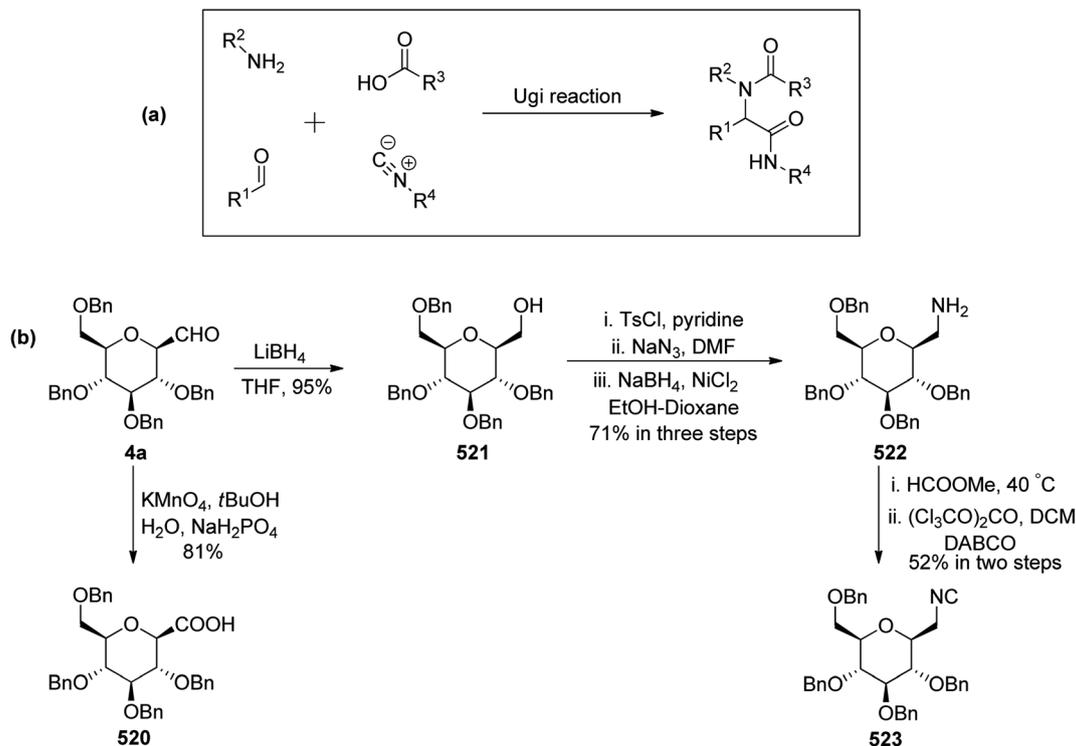
Scheme 77 Synthesis of sugar-based building blocks for the Ugi reaction, *i.e.* acid **520**, amine **522**, and isocyanide **523**.Table 4 Various sugar-based bis-amides synthesized<sup>a</sup>
