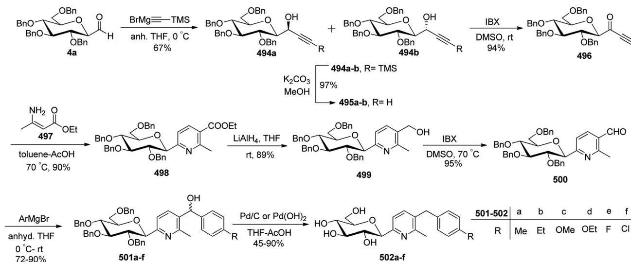
Scheme 74 Synthesis of 2- $\beta$ -D-glucopyranosyl pyridines **502a–f**.
