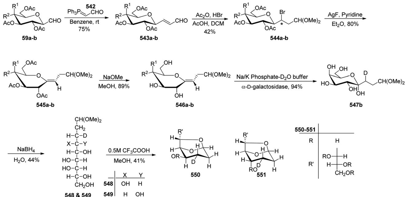
Scheme 83 Synthesis of 1,6-anhydro-2,3-dideoxy-3(S)-D-glycero-L-gluco-(3-2H)nonopyranose 550 and 551.
