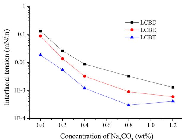
Fig. 8 Effect of Na<sub>2</sub>CO<sub>3</sub> concentration on the IFT between LCBS surfactants and Huabei crude oil at 54 °C.
