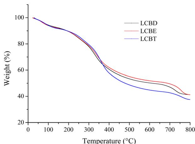
Fig. 2 TG graph of lignin carboxyl betaine.
