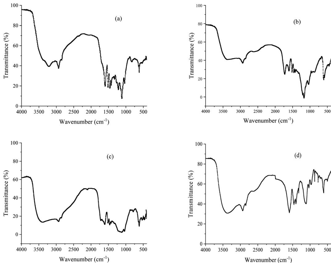
Fig. 1 FT-IR spectra of alkali lignin (a), epoxidized lignin (b), aminated lignin (c) and lignin carboxyl betaine (d).
