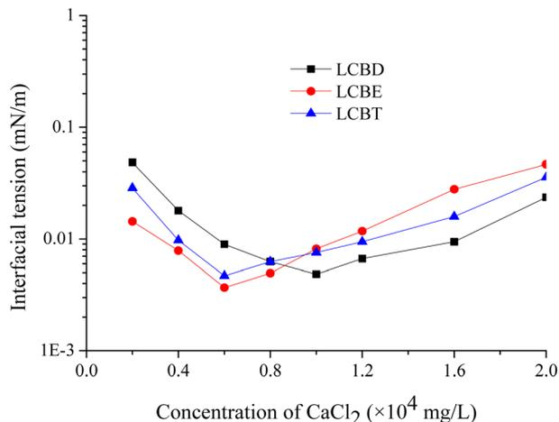
Fig. 7 Effect of CaCl<sub>2</sub> concentration on the IFT between LCBS surfactants and Huabei crude oil at 54 °C.
