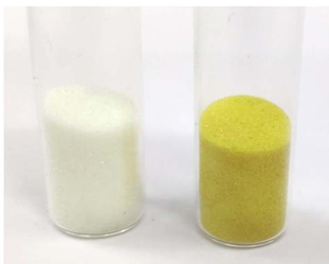
Fig. 16 Colorimetric reaction of DAS (50  $\mu\text{M}$  in MeOH) towards Ni<sup>2+</sup> in solid state.
