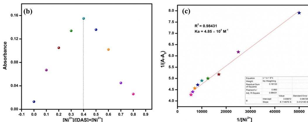
Fig. 4 (a) Absorption spectra of DAS ( $20 \mu\text{M}$ ) on sequential addition of  $\text{Ni}^{2+}$  (0– $20 \mu\text{M}$ ). (b) Job's Plot for UV-vis studies of DAS with  $\text{Ni}^{2+}$  in MeOH-PBS (5 : 1 v/v, 10 mM, pH = 7.4). (c) B-H Plot for UV-vis studies of DAS with  $\text{Ni}^{2+}$  in MeOH-PBS (5 : 1, v/v, 10 mM, pH = 7.4).
