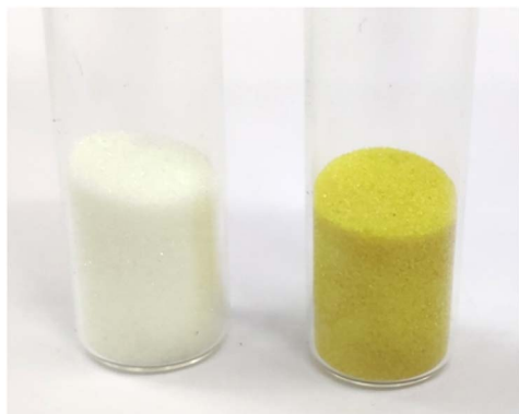
Fig. 16 Colorimetric reaction of DAS (50 \mu\text{M} in MeOH) towards Ni 2+ in solid state.
