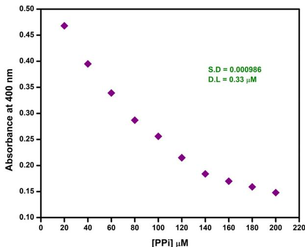
Fig. 15 Detection Limit of DAS-Ni<sup>2+</sup> ensemble for PPI.
