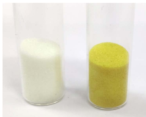
Fig. 16 Colorimetric reaction of DAS (50 \mu\text{M} in MeOH) towards \text{Ni}^{2+} in solid state.
