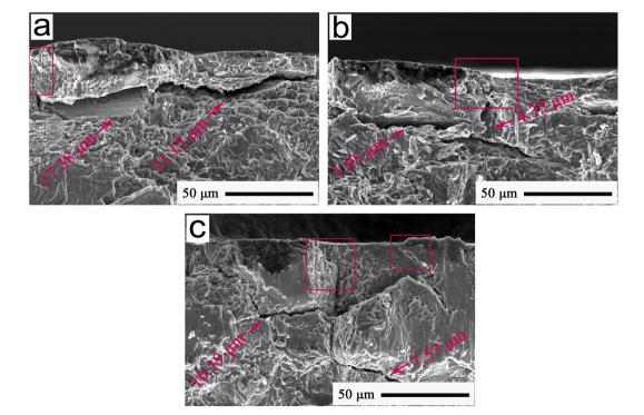
Fig. 14 FESEM cross-section images at 12 N showing the typical wear morphologies at 420 °C of (a) Ti-MA-GRa, (b) Ti-MA-GNs, and (c) Ti-MA-CNTs.
