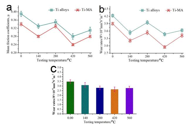
Fig. 6 (a) Typical friction coefficients and (b) wear rates for 80 min under different temperatures of the Ti alloys and Ti-MA samples; (c) mean wear rates of spherical  $Si_3N_4$  sliding against the Ti-MA.
