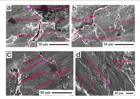
Fig. 13 FESEM images showing the typical morphologies for 80 min of friction interfaces at 420 °C and 12 N of (a) Ti-MA-GRa, (b) Ti-MA-GNs, and (c) Ti-MA-CNTs; (d) interface morphology of spherical  $Si_3N_4$  sliding against the Ti-MA-CNTs.
