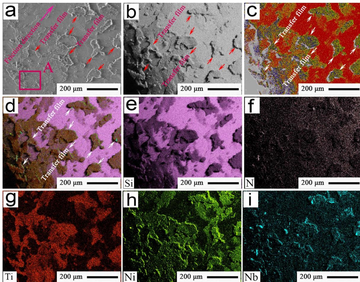
Fig. 8 Typical FESEM morphology (a), backscattered electron image (b), mapping patterns (c) and (d), and main element distributions (e)–(i) of the friction interface at 420 °C of the spherical  $\text{Si}_3\text{N}_4$  sliding against the Ti alloys.
