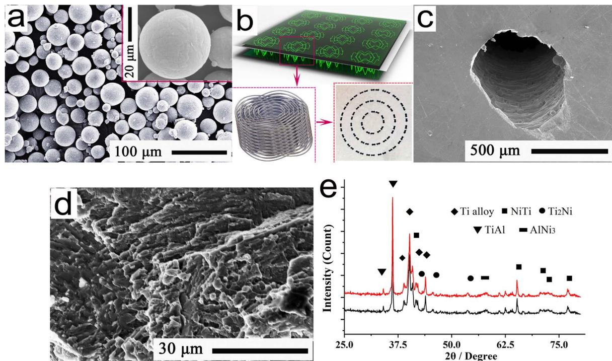
Fig. 1 (a) Typical EPMA pattern of the spherical powders; (b) morphologies of the sinusoidal micropores; (c) FESEM image of the single micropore; (d) cross-section morphology; (e) XRD diffraction pattern of Ti alloy.
