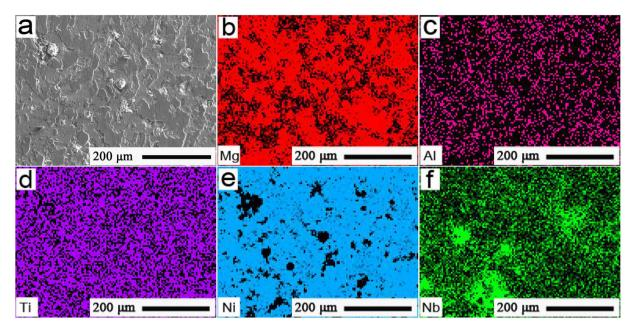
Fig. 10 (a) EPMA images showing the typical wear morphology and (b)-(f) main element distributions at 280 °C and 12 N of the friction interfaces.
