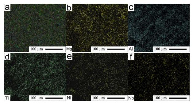
Fig. 3 (a) Typical mapping pattern and (b)-(f) FESEM distributions of the primary elements of the interface microchannel presented in Fig. 2c.
