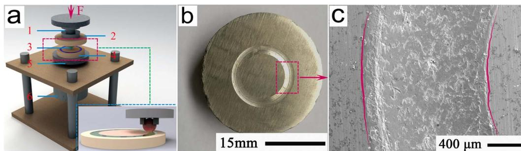
Fig. 4 (a) Typical schematic of the ball-on-disk tribopair system; inset shows the frictional contact between the  $\text{Si}_3\text{N}_4$  ball and the disk sample indicated by the dotted rectangle; (b) and (c) typical morphologies of the frictional interfaces.
