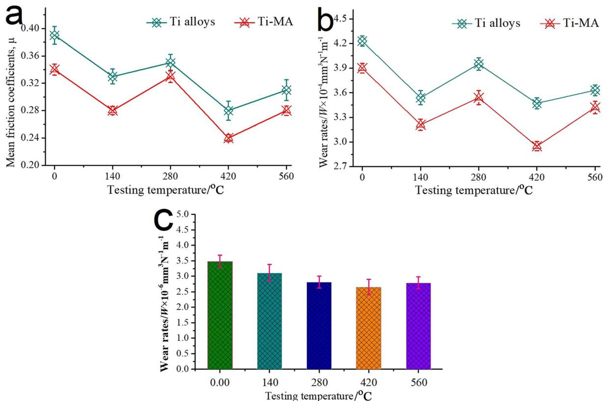
Fig. 6 (a) Typical friction coefficients and (b) wear rates for 80 min under different temperatures of the Ti alloys and Ti-MA samples; (c) mean wear rates of spherical  $\text{Si}_3\text{N}_4$  sliding against the Ti-MA.
