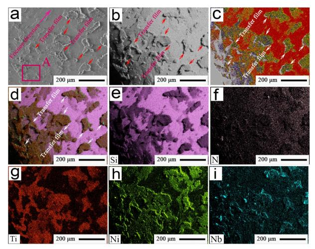
Fig. 8 Typical FESEM morphology (a), backscattered electron image (b), mapping patterns (c) and (d), and main element distributions (e) – (i) of the friction interface at 420 °C of the spherical Si<sub>3</sub>N<sub>4</sub> sliding against the Ti alloys.
