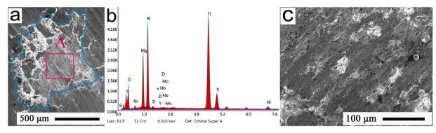
Fig. 2 (a) Typical FESEM morphology of the single microchannel; (b) EDS spectrum of the material in (a), (c) amplified morphology of the region bounded by the red rectangle A in (a).
