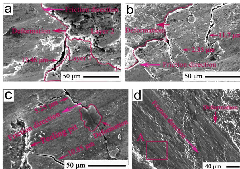
Fig. 13 FESEM images showing the typical morphologies for 80 min of friction interfaces at 420 °C and 12 N of (a) Ti-MA-GRa, (b) Ti-MA-GNs, and (c) Ti-MA-CNTs; (d) interface morphology of spherical  $\text{Si}_3\text{N}_4$  sliding against the Ti-MA-CNTs.
