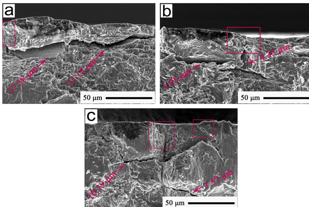
**Fig. 14** FESEM cross-section images at 12 N showing the typical wear morphologies at 420 °C of (a) Ti-MA-GRa, (b) Ti-MA-GNs, and (c) Ti-MA-CNTs.
