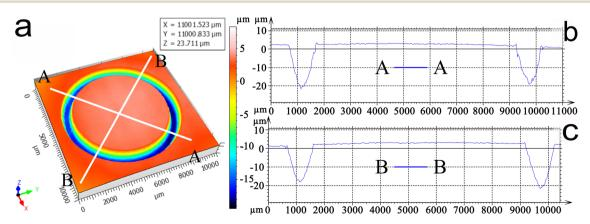
Fig. 5 (a) Typical 3D pattern of the wear profile, and (b) and (c) 2D wear profiles extracted from the straight lines AA and BB of Fig. 5b.
