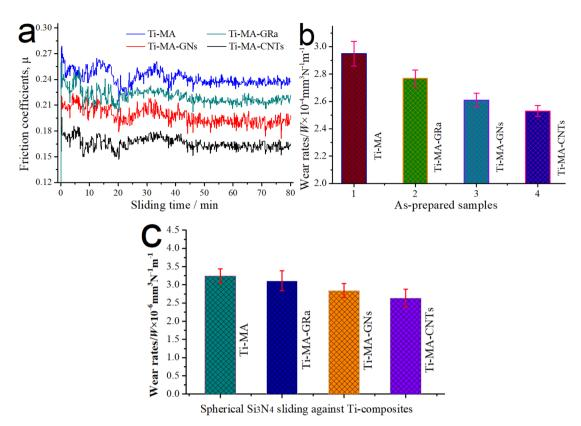
Fig. 12 (a) Typical friction coefficients and (b) wear rates at 420 °C and 12 N for Ti-MA, Ti-MA-GRa, Ti-MA-GNs, and Ti-MA-CNTs; (c) mean wear rates of the spherical  $Si_3N_4$ .
