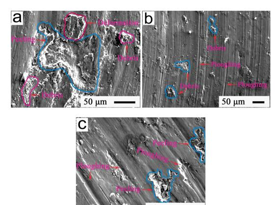
Fig. 7 EPMA patterns indicating the typical wear morphologies after 80 min for friction interfaces of pure Ti-alloys at (a) 280 °C, (b) 420 °C, and (c) 560 °C.
