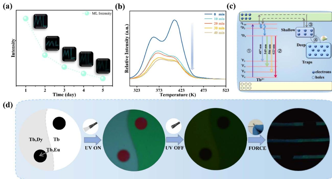
Fig. 5 (a) ML intensity of SGO:0.005Tb<sup>3+</sup>, 0.004Dy<sup>3+</sup> recorded after deposited in air for 1, 2, 3, 4, and 5 days; (b) time-dependent TL curves of SGO:0.005Tb<sup>3+</sup>, 0.004Dy<sup>3+</sup> under 5 N load after UV irradiation 20 min; (c) luminescence diagram of SGO:Tb<sup>3+</sup>, Dy<sup>3+</sup>; (d) the photo of the anti-counterfeiting based on the as-obtained SGO:Tb<sup>3+</sup>, SGO:Tb<sup>3+</sup>, Dy<sup>3+</sup> and SGO:Tb<sup>3+</sup>, Eu<sup>3+</sup>.
