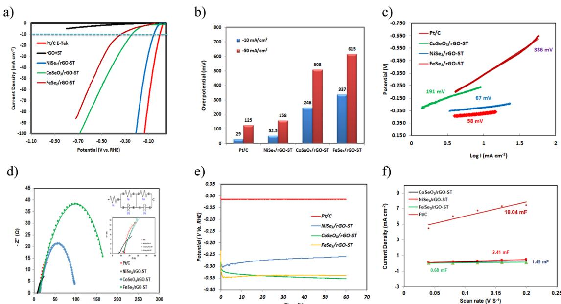
Fig. 5 OER performance of the electrocatalysts Pt/C E-TEK,  $\text{NiSe}_2/\text{rGO-ST}$ ,  $\text{CoSeO}_3/\text{rGO-ST}$  and  $\text{FeSe}_2/\text{rGO-ST}$ . (a) LSV curves, (b) the comparison of the overpotential, (c) Tafel plots derived from LSV curves, (d) Nyquist plots, (e) chronopotentiometry (CP) curve, and (f) the double-layer capacitance ( $C_{dl}$ ) plots.
