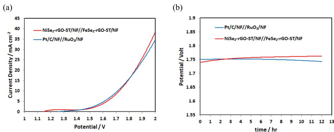
Fig. 7 (a) LSV curves of Pt/C/NF||RuO<sub>2</sub>/NF and NiSe<sub>2</sub>-rGO-ST/NF||FeSe<sub>2</sub>-rGO-ST/NF, (b) the chronoamperometry curve of Pt/C/NF||RuO<sub>2</sub>/NF and NiSe<sub>2</sub>-rGO-ST/NF||FeSe<sub>2</sub>-rGO-ST/NF at 10 mA cm<sup>-2</sup>.
