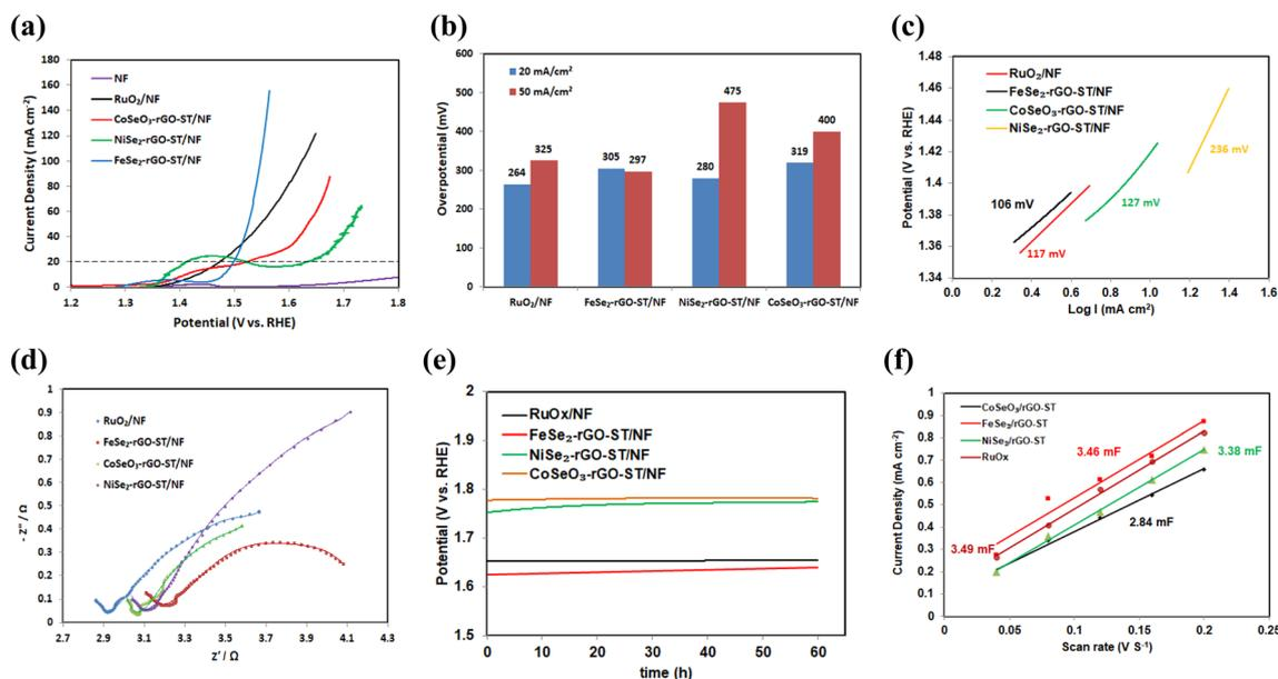
Fig. 6 OER performance of the electrocatalysts  $RuO_x$ ,  $NiSe_2/rGO-ST$ ,  $CoSeO_3/rGO-ST$ , and  $FeSe_2/rGO-ST$ . (a) LSV curves, (b) the comparison of the overpotential, (c) Tafel plots derived from LSV curves, (d) Nyquist plots, and (e) chronopotentiometry (CP) curve at  $30\text{ mA cm}^{-2}$ .
