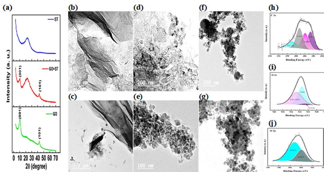
Fig. 1 (a) XRD pattern of ST, rGO and rGO-ST, HR-TEM images of the GO (b and c), silica template (d and e), and rGO-ST (f and g), high-resolution XPS spectra of the C 1s (h), O 1s (i), and Si 2p (j) on the surface of the mixed support rGO-ST.
