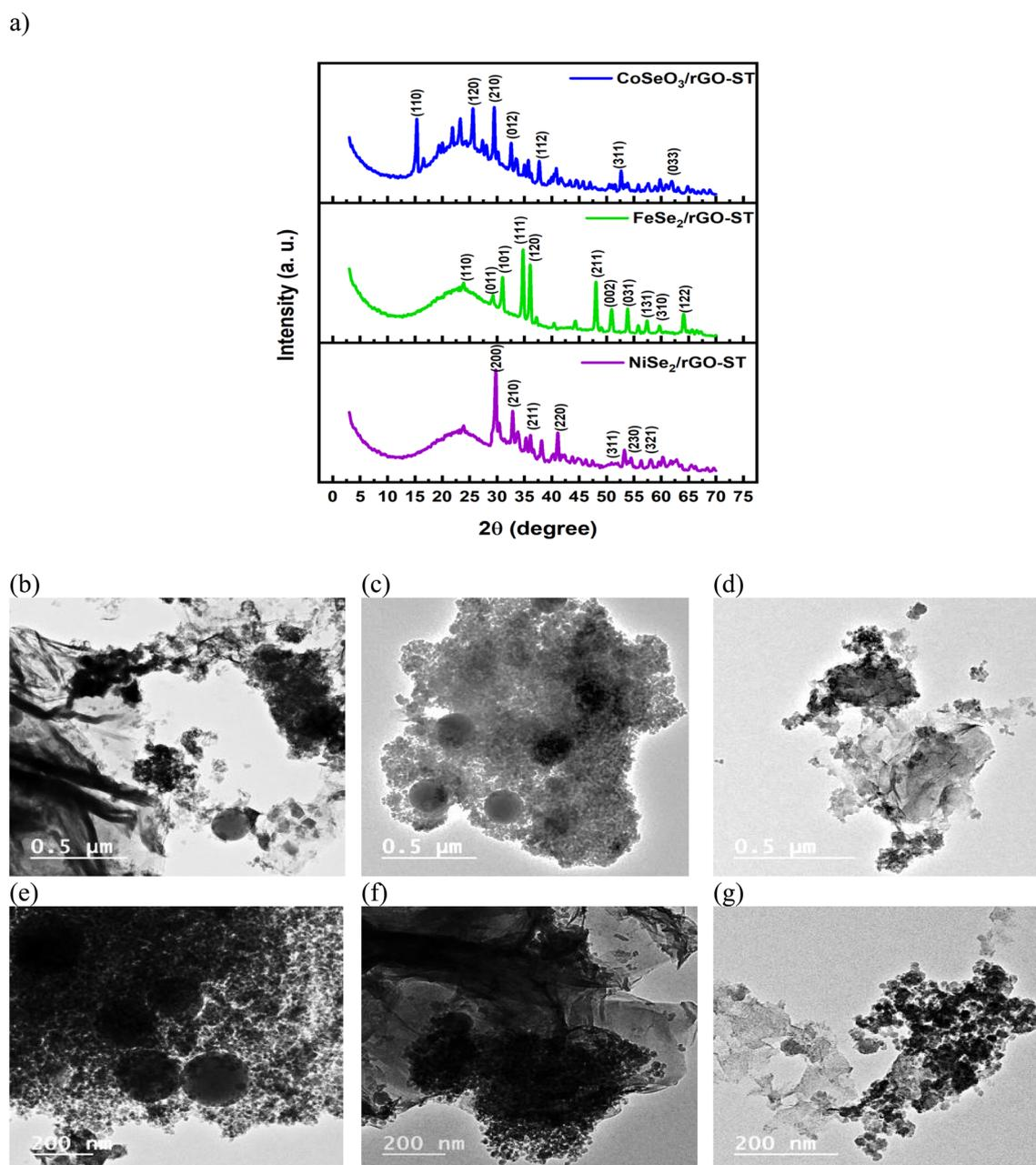
Fig. 2 XRD analysis of the electrocatalyst (a), HR-TEM analysis of NiSe<sub>2</sub>/rGO-ST (b and c), CoSe<sub>3</sub>/rGO-ST (d and e), and FeSe<sub>2</sub>/rGO-ST (f and g).
