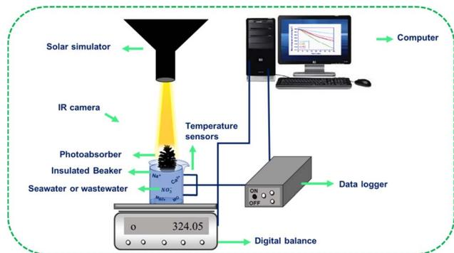
Fig. 2 Schematic representation of the ISSG setup.
