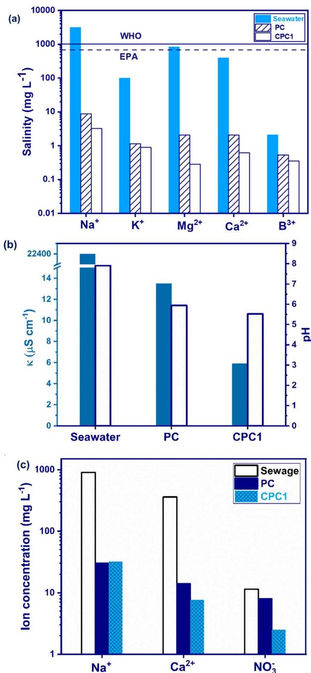
Fig. 7 (a) Concentration of various ions, and (b)  $\kappa$  and pH of the seawater before and after desalination by PC and CPC1. The filled and unfilled bars represent the electrical conductivity and pH, respectively. (c) The ion concentrations of the sewage before and after purification by PC and CPC1.
