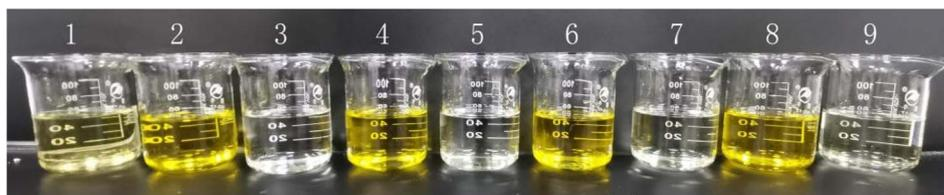
Fig. 9 Decolorization effect of 200D, 400D, 600D, and 800D NFs on the raw synthetic solution. Number 1 is the raw synthetic solution, numbers 2, 4, 6, and 8 are the concentrated solutions of 200D, 400D, 600D, and 800DNFs, numbers 3, 5, 7, and 9 are the permeate solutions of 200D, 400D, 600D, and 800D NFs
