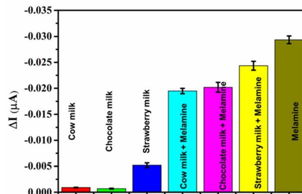
**Fig. 8** Responses of the CuO/MIP electrode in real samples, namely, cow milk, chocolate milk, strawberry milk, melamine-contaminated cow milk, melamine-contaminated chocolate milk, melamine-contaminated strawberry milk, and melamine.
