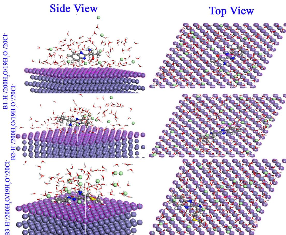
Fig. 16 Monte Carlo simulations for the most favorable modes of adsorption obtained for B1-H<sup>+</sup>, B2-H<sup>+</sup> and B3-H<sup>+</sup> on Fe (110) surface, side and top view.
