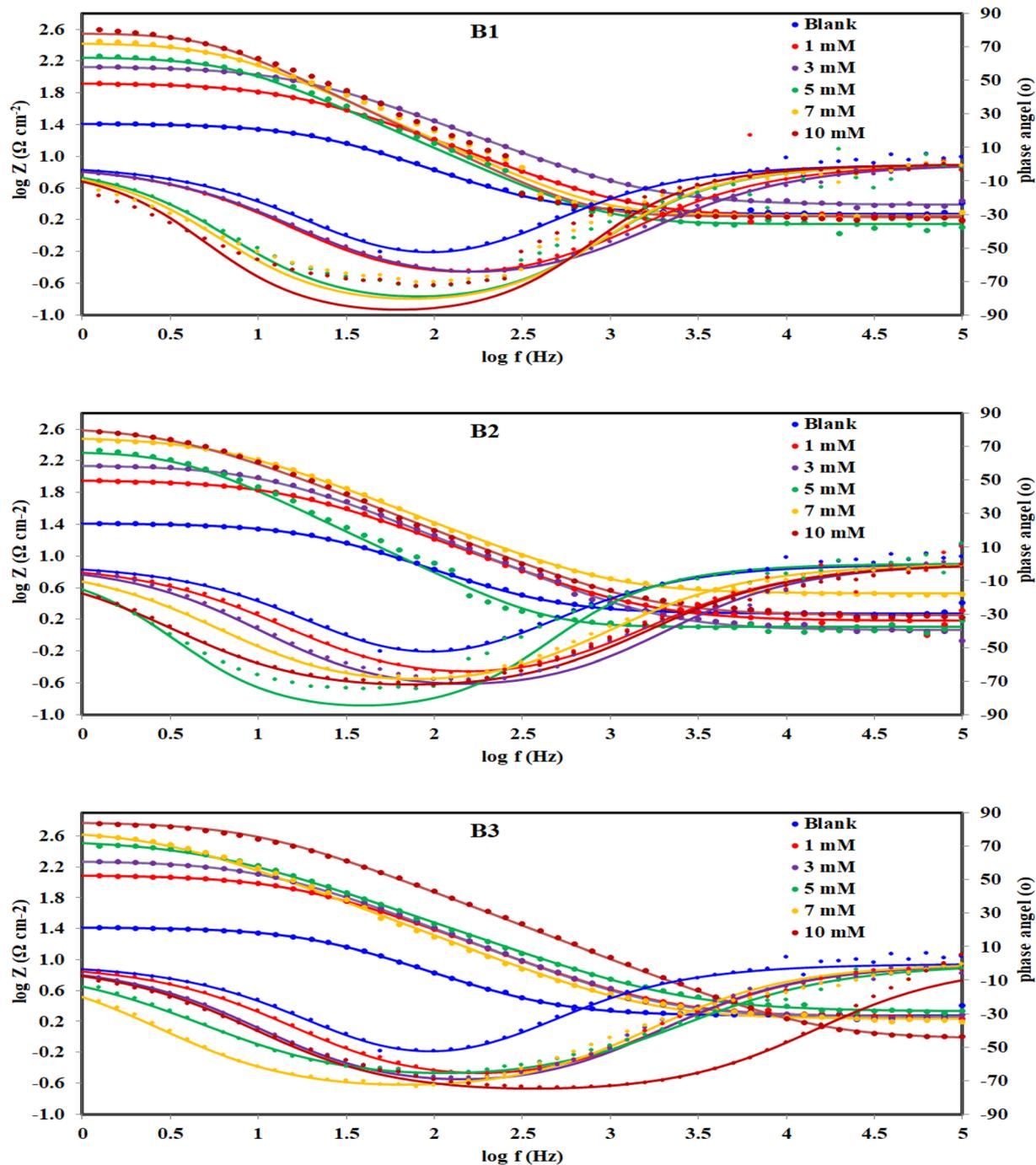
Fig. 9 Bode and phase angle plots for c-steel in 1.0 M HCl solution without and with different concentrations of B1, B2 and B3 compounds at 30 °C.
