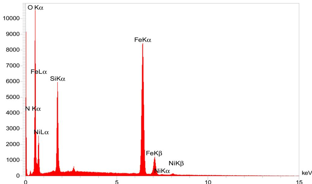
Fig. 2 EDX spectrum of Ni<sup>II</sup>-picolylamine/TCT/APTES@SiO<sub>2</sub>@Fe<sub>3</sub>O<sub>4</sub> catalyst.
