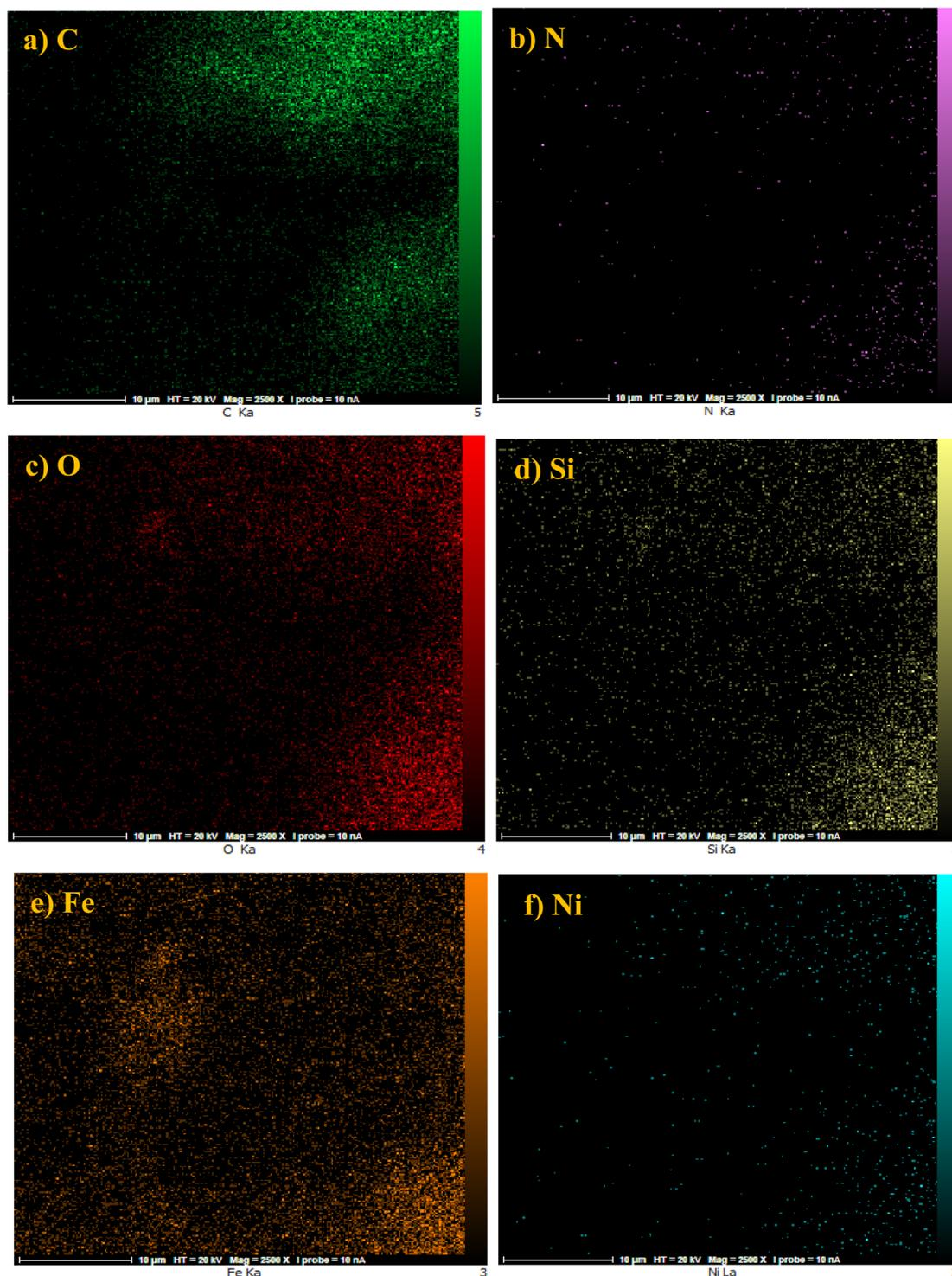
Fig. 3 Elemental mapping analysis of Ni<sup>II</sup>-picolylamine/TCT/APTES@SiO<sub>2</sub>@Fe<sub>3</sub>O<sub>4</sub> catalyst: (a) C, (b) N, (c) O, (d) Si, (e) Fe, and (f) Ni.
