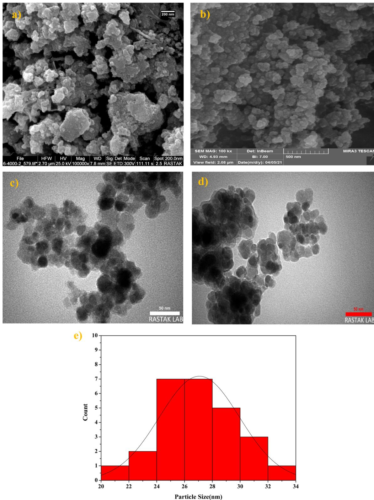
Fig. 8 FE-SEM of (a) Fe<sub>3</sub>O<sub>4</sub>, (b) Ni<sup>II</sup>-picolylamine/TCT/APTES@SiO<sub>2</sub>@Fe<sub>3</sub>O<sub>4</sub>, TEM of (c) Fe<sub>3</sub>O<sub>4</sub>, (d) Ni<sup>II</sup>-picolylamine/TCT/APTES@SiO<sub>2</sub>@Fe<sub>3</sub>O<sub>4</sub>, and (e) size distribution of Ni<sup>II</sup>-picolylamine/TCT/APTES@SiO<sub>2</sub>@Fe<sub>3</sub>O<sub>4</sub>.
