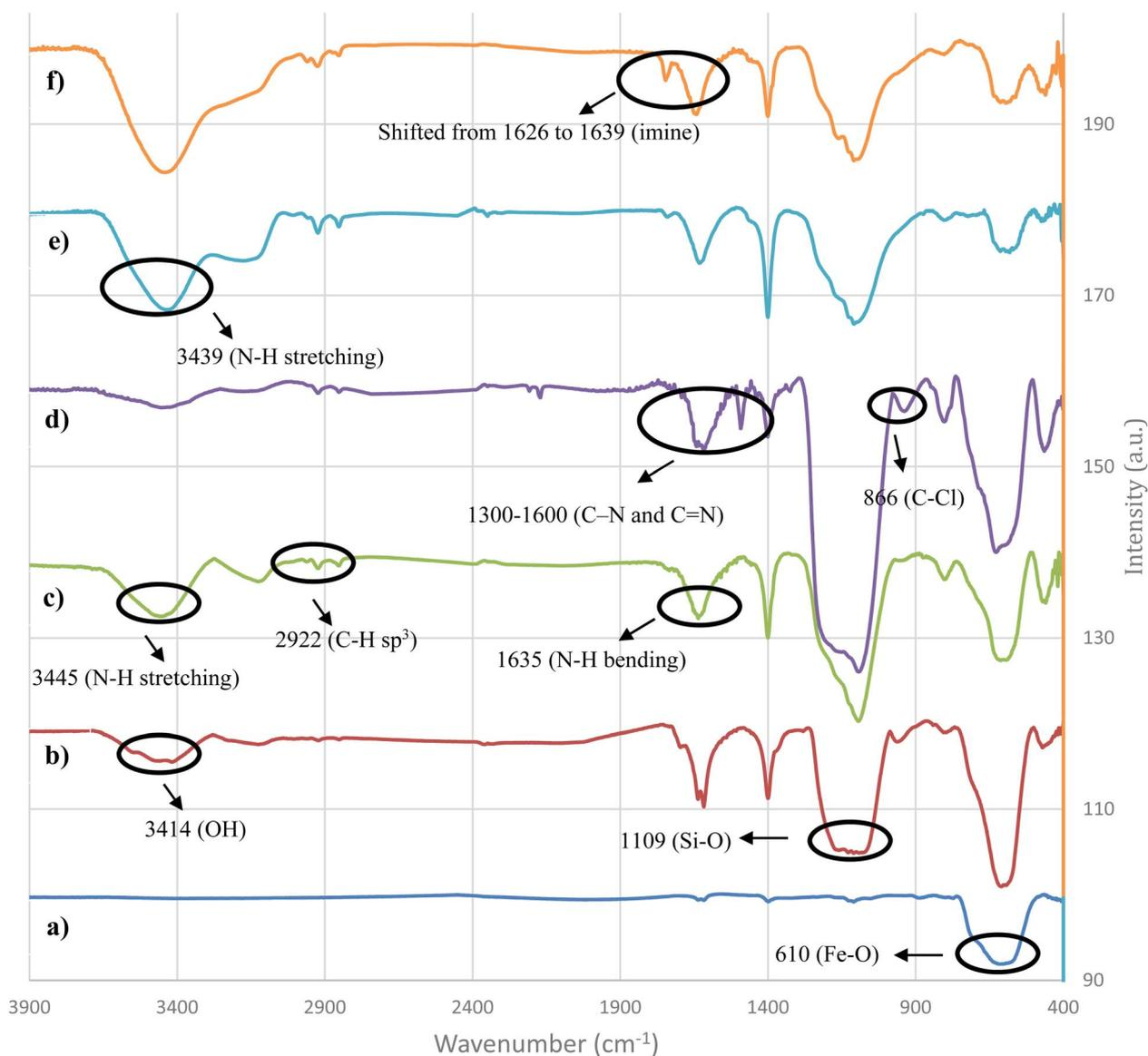
Fig. 1 FT-IR spectra of (a) Fe<sub>3</sub>O<sub>4</sub>, (b) SiO<sub>2</sub>@Fe<sub>3</sub>O<sub>4</sub>, (c) APTES@SiO<sub>2</sub>@Fe<sub>3</sub>O<sub>4</sub>, (d) TCT/APTES@SiO<sub>2</sub>@Fe<sub>3</sub>O<sub>4</sub>, (e) picolylamine/TCT/APTES@SiO<sub>2</sub>@Fe<sub>3</sub>O<sub>4</sub>, and (f) Ni<sup>II</sup>-picolylamine/TCT/APTES@SiO<sub>2</sub>@Fe<sub>3</sub>O<sub>4</sub>.
