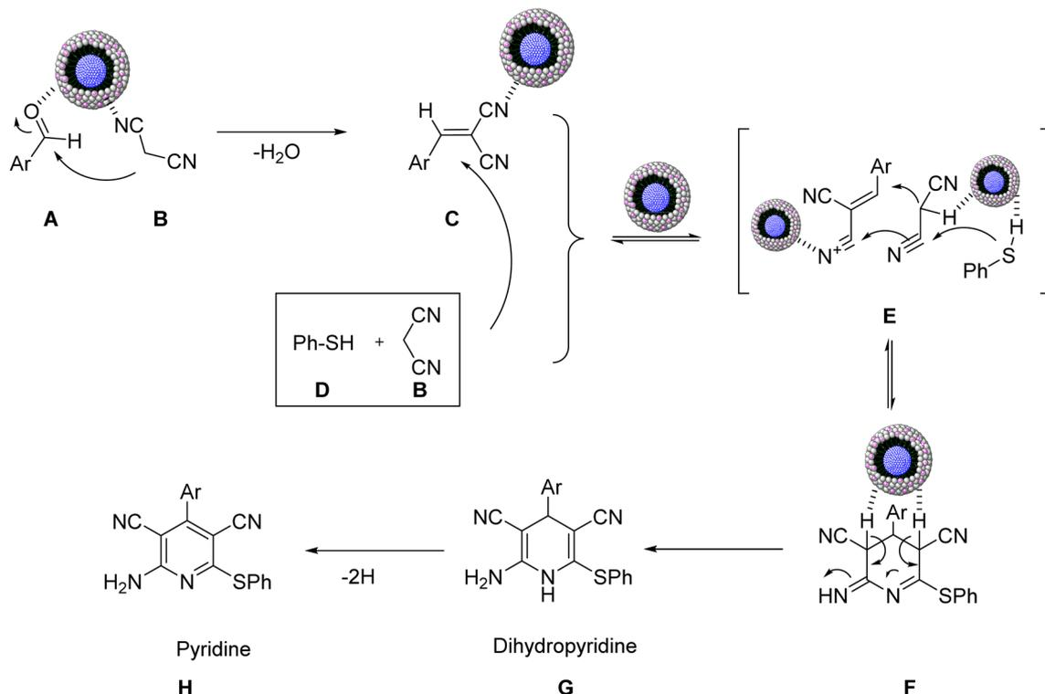
Scheme 6 Plausible mechanism for the construction of substituted pyridine derivatives catalyzed by Ni<sup>II</sup>-picolylamine/TCT/APTES@SiO<sub>2</sub>@Fe<sub>3</sub>O<sub>4</sub>.
