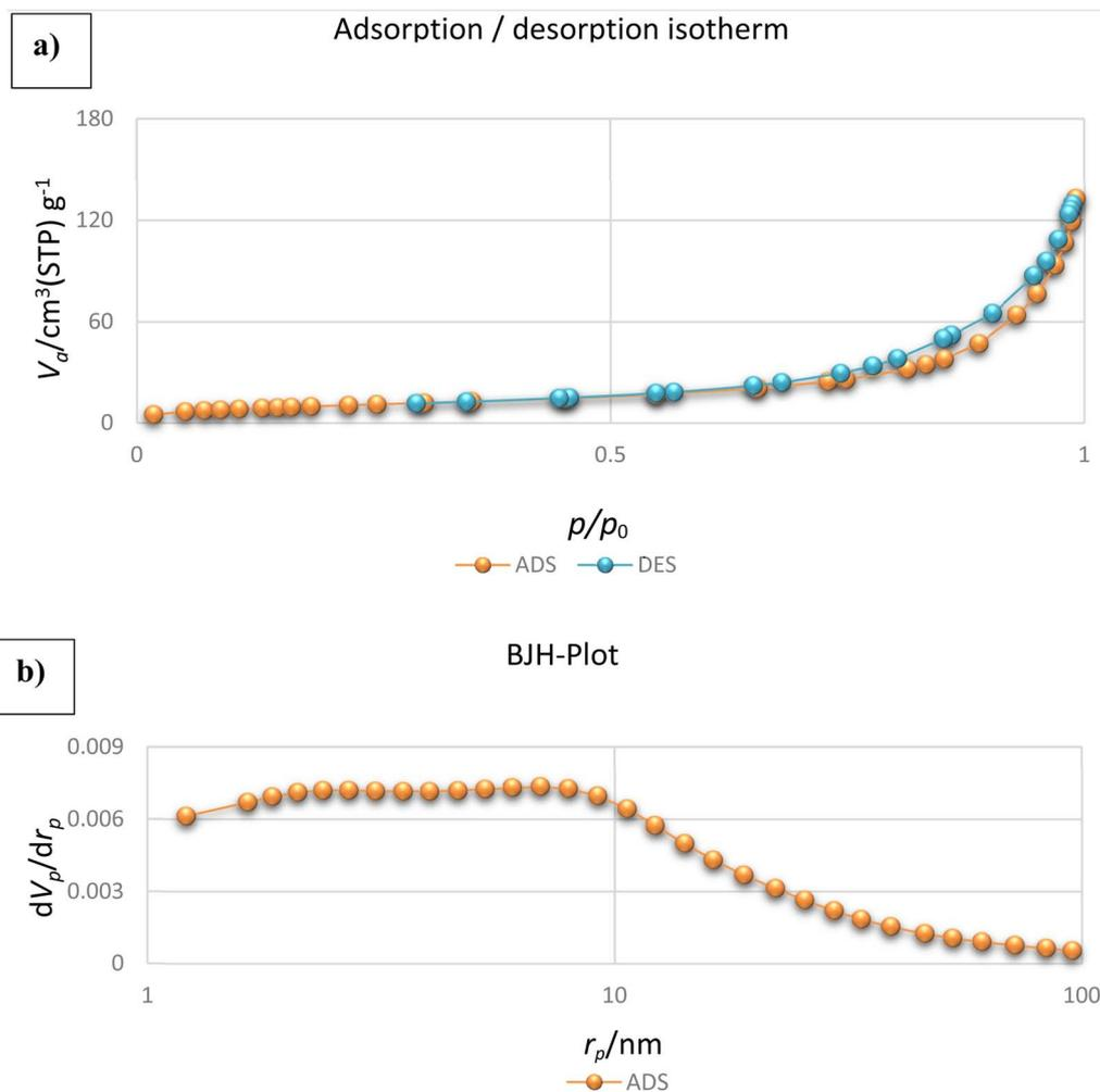
Fig. 9 (a) BET plot of the nitrogen adsorption–desorption and (b) pore-size distribution curve of the Ni<sup>II</sup>-picolyamine/TCT/APTES@SiO<sub>2</sub>@Fe<sub>3</sub>O<sub>4</sub>.
