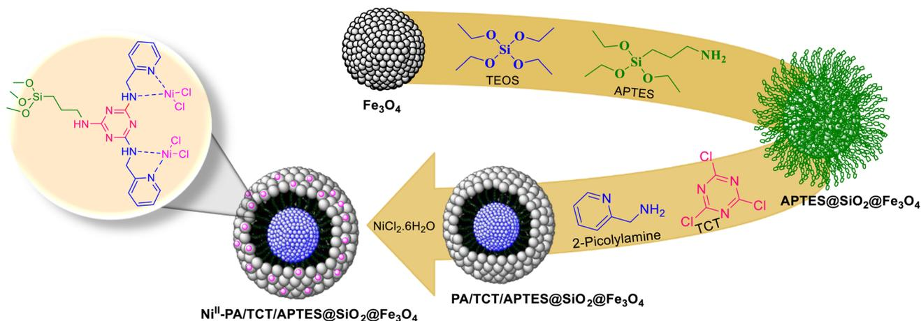
Scheme 4 Preparation of the Ni<sup>II</sup>-picolylamine/TCT/APTES@SiO<sub>2</sub>@Fe<sub>3</sub>O<sub>4</sub> catalyst.
