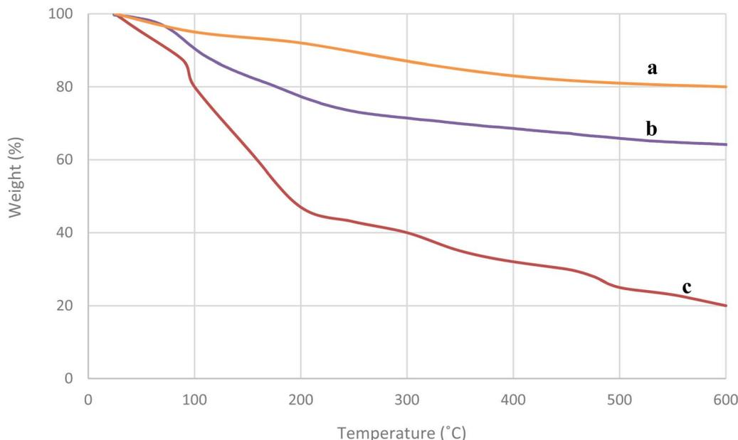
Fig. 7 TGA analysis of (a) Fe<sub>3</sub>O<sub>4</sub>, (b) SiO<sub>2</sub>@Fe<sub>3</sub>O<sub>4</sub>, and (c) Ni<sup>II</sup>-picolylamine/TCT/APTES@SiO<sub>2</sub>@Fe<sub>3</sub>O<sub>4</sub>.
