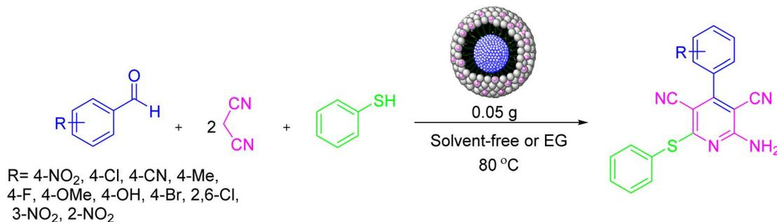
Scheme 3 Activity of the Ni<sup>II</sup>-picolyamine/TCT/APTES@SiO<sub>2</sub>@Fe<sub>3</sub>O<sub>4</sub> catalyst for the synthesis of substituted pyridine derivatives.
