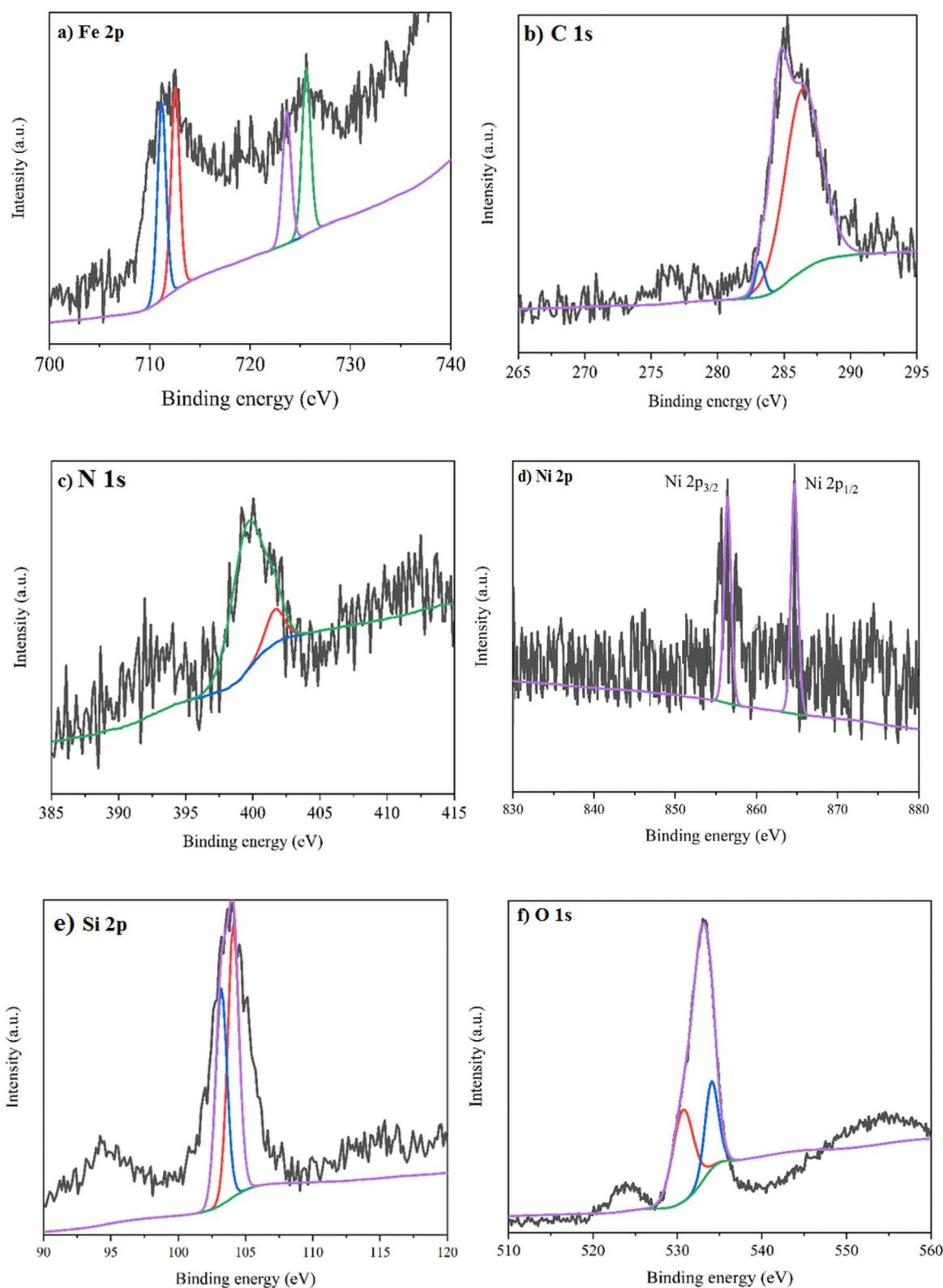
Fig. 4 XPS spectra of Ni<sup>II</sup>-picolylamine/TCT/APTES@SiO<sub>2</sub>@Fe<sub>3</sub>O<sub>4</sub> catalyst: (a) Fe 2p, (b) C 1s, (c) N 1s, (d) Ni 2p, (e) Si 2p, and (f) O 1s.
