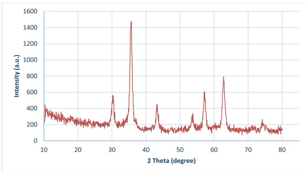
Fig. 5 XRD patterns of Ni<sup>II</sup>-picolylamine/TCT/APTES@SiO<sub>2</sub>@Fe<sub>3</sub>O<sub>4</sub> catalyst.
