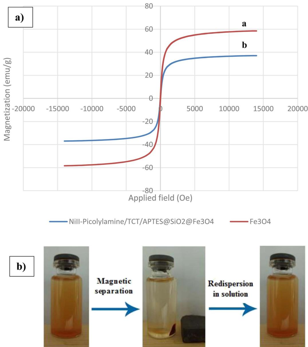
Fig. 6 (a) VSM analysis, (b) image of the magnetic separation and redispersion of Ni<sup>II</sup>-picolylamine/TCT/APTES@SiO<sub>2</sub>@Fe<sub>3</sub>O<sub>4</sub>.
