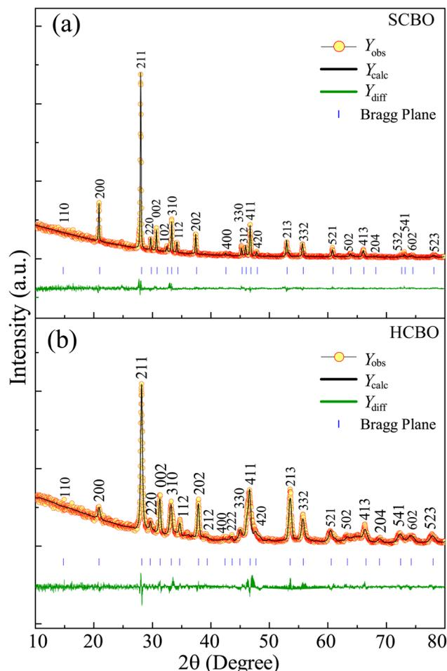
Fig. 2 Rietveld refined XRD patterns on top of experimentally observed data of (a) SCBO and (b) HCBO. The yellow circles are the experimental data points ( $Y_{obs}$ ), the black solid line represents the calculated refined pattern  $Y_{calc}$ , the bottom green curve  $Y_{diff}$  shows the difference between the experimental  $Y_{obs}$  and calculated  $Y_{calc}$  values.
