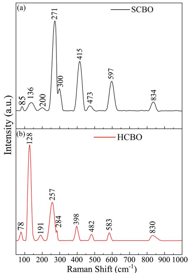
Fig. 5 RT Raman spectra of (a) SCBO, (b) HCBO samples.
