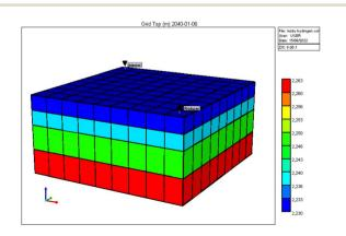
Fig. 4 Reservoir grid layout generated by CMG STARS.
