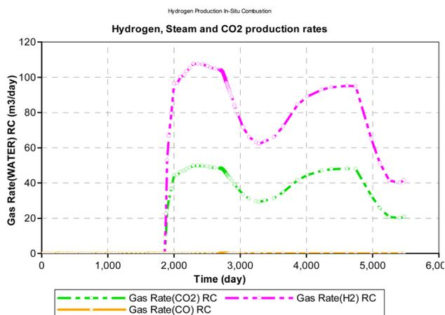
Fig. 16 Effect of OC on H<sub>2</sub>, CO<sub>2</sub>, CO production rate (CMG STARS).
