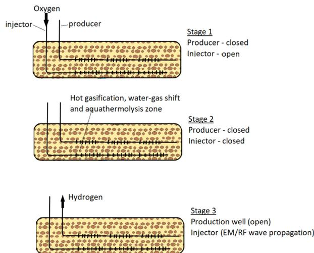
Fig. 1 *In situ* hydrogen production process adapted from (Gates & Wang, 2017).<sup>1</sup>
