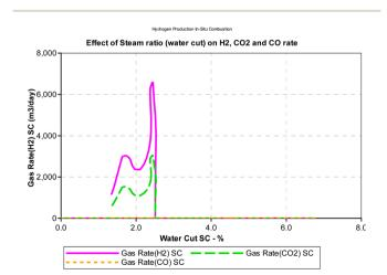
Fig. 14 Effect of SC on H<sub>2</sub>/CO/CO<sub>2</sub> production rates (CMG STARS).
