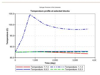
Fig. 11 Change in temperature during combustion at select points on the reservoir grid (at atmospheric pressure).
