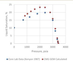
Fig. 8 Constant volume depletion analysis.
