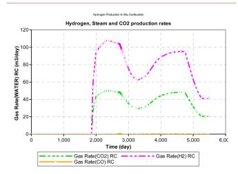
Fig. 16 Effect of OC on H<sub>2</sub>, CO<sub>2</sub>, CO production rate (CMG STARS).
