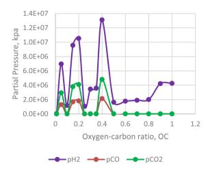
Fig. 15 Effect of oxygen-carbon ratio on H<sub>2</sub>/CO/CO<sub>2</sub> production.
