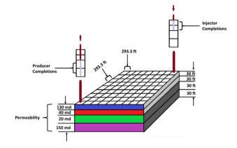
Fig. 3 Reservoir grid model based on Kenyon (1987).20
