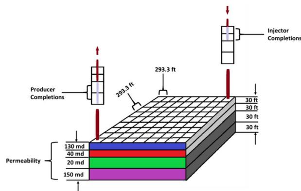
Fig. 3 Reservoir grid model based on Kenyon (1987).<sup>20</sup>
