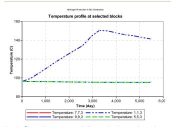
Fig. 12 Change in temperature during combustion at select points on the reservoir grid (at reservoir pressure).
