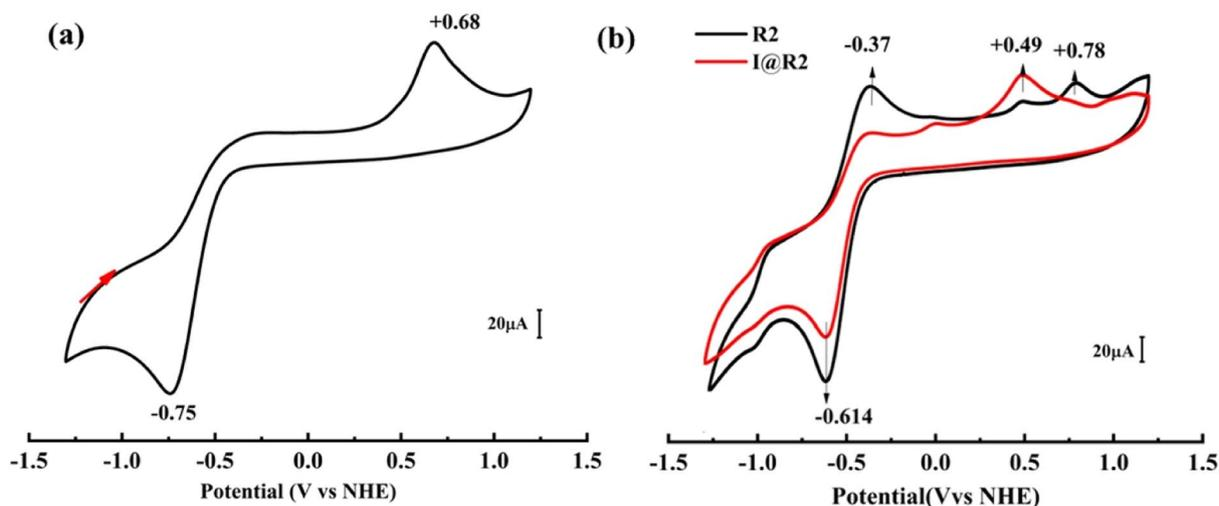
Fig. 2 (a) CV measurements of clusters I; the arrows indicate the scan direction. (b) CV measurements of R2 and I@R2.
