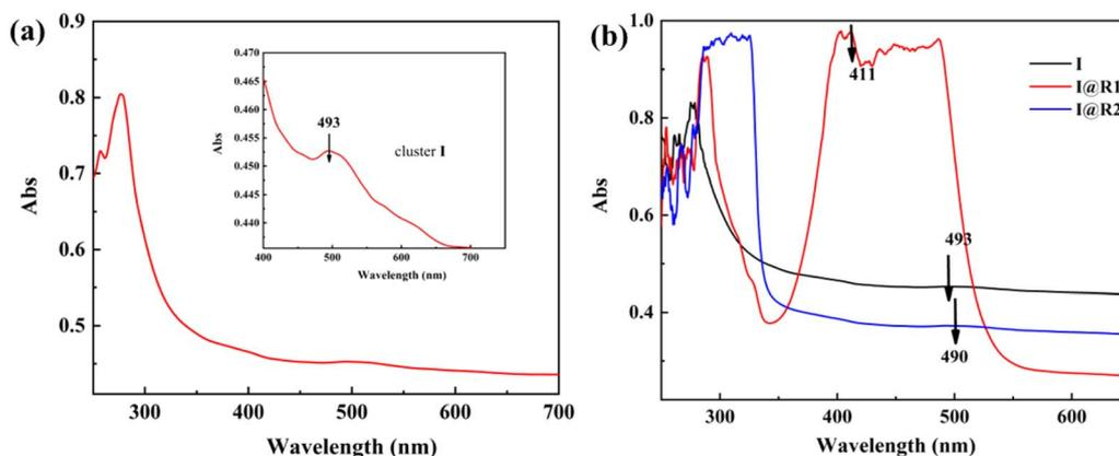
Fig. 4 (a) UV-vis absorption spectrum of 20  $\mu\text{M}$  clusters **I** in PO (Inset is the enlarged spectrum of clusters **I** in the visible region). (b) UV-vis absorption spectra of **I** (black), **I@R1** (red) and **I@R2** (blue) in PO.
