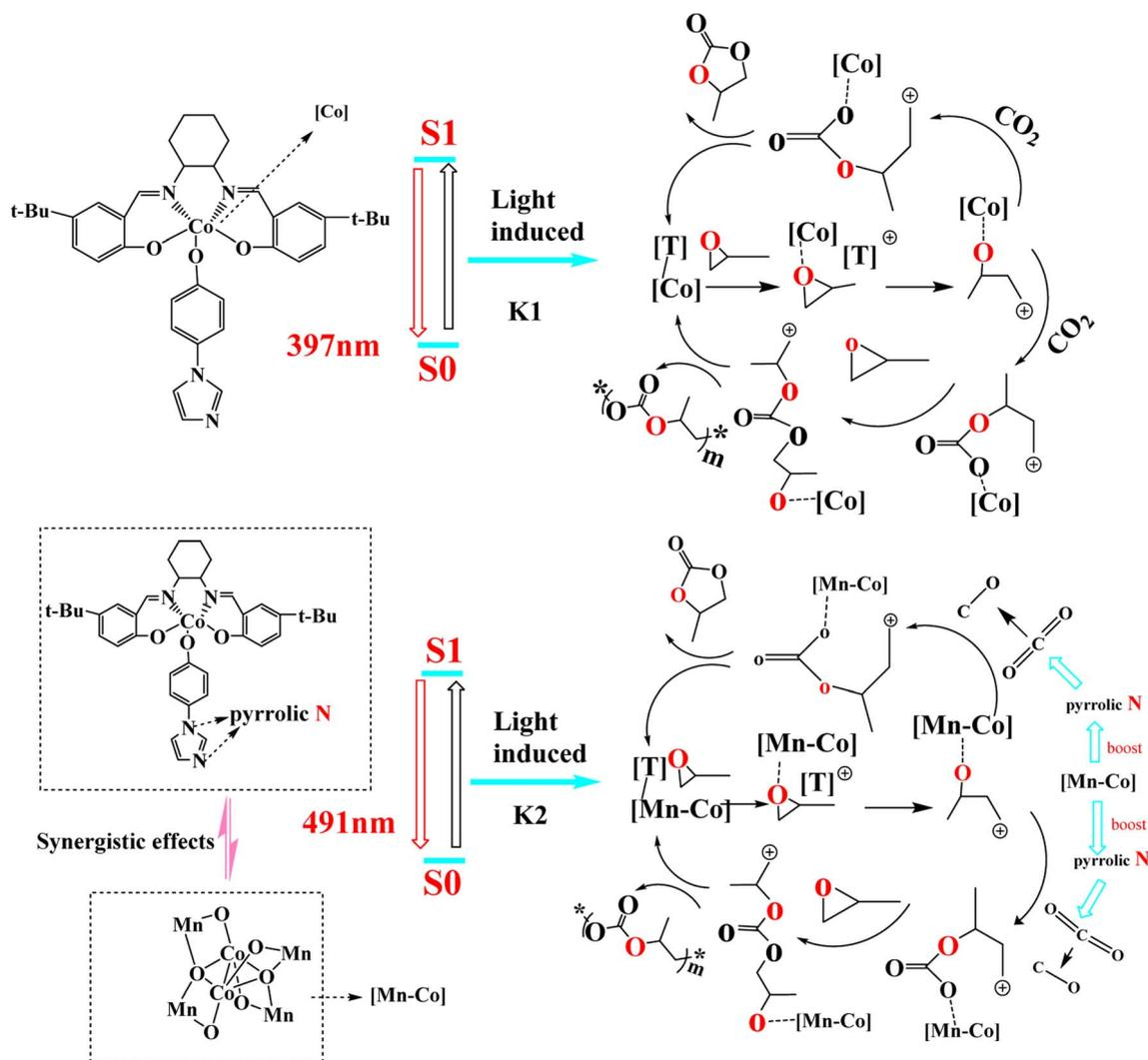
Scheme 3 S1 and I@S1 catalytic copolymerization mechanism of carbon dioxide and PO.
