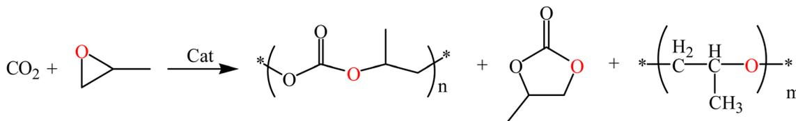
Scheme 1 Copolymerization route: CO<sub>2</sub> and PO copolymerization catalyzed by a catalyst.
