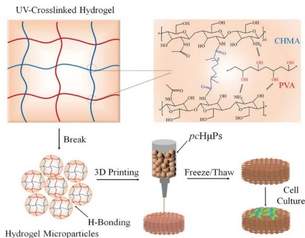
Fig. 5 Schematic illustration to the preparation of the self-healing pre-cross-linked hydrogel microparticles (pcH $\mu$ Ps) by 3D printing for cell spheroid growth.<sup>199</sup> Reproduced from ref. 199 with permission from Wiley, copyright 2020.
