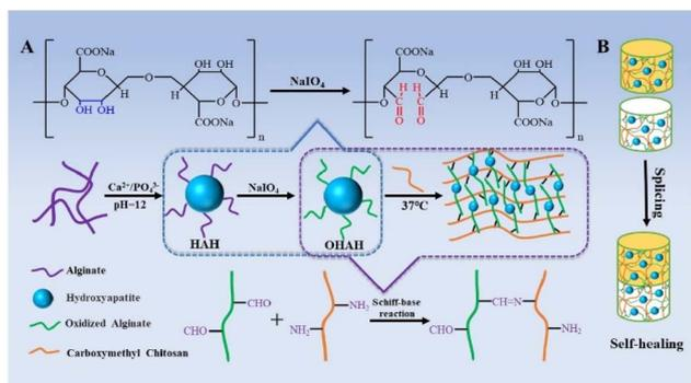
Fig. 3 Schematic illustration (A) of the preparation of injectable hydrogels *via* Schiff base reaction. (B) The self-healing property of the hydrogels.<sup>183</sup> Reproduced from ref. 183 with permission from Elsevier, copyright 2020.
