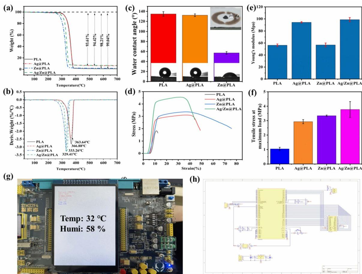
Fig. 2 (a) Thermogram and (b) DTG curves of PLA, Ag@PLA, Zn@PLA, and Ag/Zn@PLA. (c) The contact angle of PLA, Ag@PLA, and Zn@PLA. (d) The stress–strain curves of PLA, Ag@PLA, and Zn@PLA. (e) Young's modulus and (f) tensile strength of PLA, Ag@PLA, and Zn@PLA. (g) Single-chip monitor displays temperature obtained by a temperature sensor. (h) Schematic circuit diagram of the dressing device.
