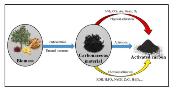
Fig. 13 Schematic illustration of the classical fabrication and activation techniques of activated carbon (this figure has been reproduced from Mariana *et al.*<sup>121</sup> with permission from Elsevier, copyright 2021).
