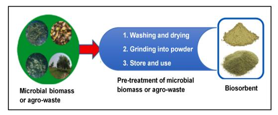
Fig. 12 A schematic diagram showing the step-by-step procedure for the preparation of the biosorbent from microbial biomass or agro-based waste (this figure has been adapted from Bilal et al.<sup>32</sup> with permission from Elsevier, copyright 2022).
