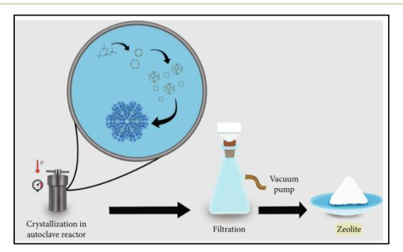
Fig. 14 A schematic diagram showing hydrothermal processes for synthesizing zeolite sorbent material for water pollutants removal (this figure has been adapted from De Magalhães *et al.*<sup>138</sup> with permission from Hindawi, copyright 2022).
