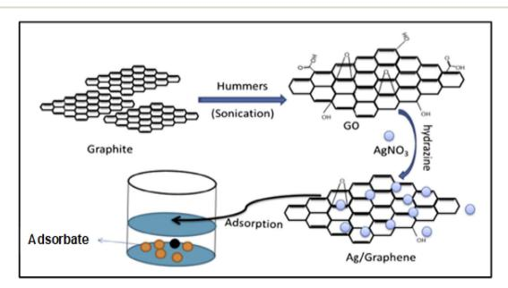
Fig. 19 A schematic diagram showing the synthesis process of graphene-based adsorbent for adsorbate molecules removal (this figure has been adapted from Qu *et al.*<sup>164</sup> with permission from Elsevier, copyright 2017).
