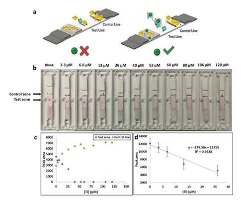
Fig. 7 (a) The adsorption and desorption method of colorimetric LFAs. (b) The LFA (AuNPs based) for Tl(i) detection with various concentrations of Tl(i) ions (ranges from  $0-120 \mu M$ ). (c) The curve was plotted against to the peak area control (c) and test (T) zones vs. various concentrations of Tl(i) were analyzed by ImageJ software. (d) Plot showing the linear dynamic range.
