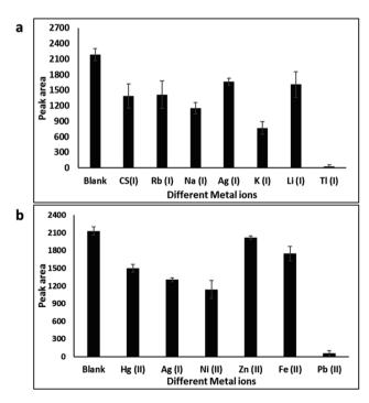
Fig. 8 (a) The AuNPs based LFA selectivity experiments for Tl(i) over K(i), Rb(i), Na(i), Cs(i), Ag(i) and Li(i). All the metal ions concentrations were 120  $\mu\text{M}$ . (b) The AuNPs based LFA selectivity experiments for Pb(ii) over Zn(ii), Ag(i), Hg(ii), Ni(ii), and Fe(ii). All the ion concentrations were 150 nM. Triplicate experiments were performed. The histogram of corresponding peak area (test (T) zone vs. various metal ions) were analyzed by ImageJ software.
