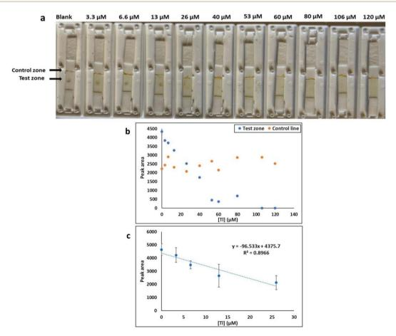
Fig. 9 (a) The LFA (AgNPs based) for Tl(i) (from 0–120  $\mu$ M). (b) The curve was plotted against the peak area of test (T) and control (C) lines vs. various Tl(i) ions concentrations and were analyzed by ImageJ software. (c) Plot of the linear dynamic range.
