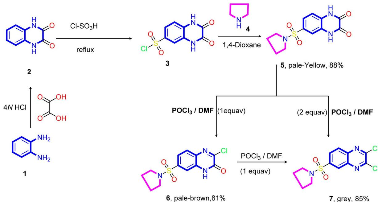
**Scheme 1** Synthetic pathways of the 2,3-dioxo-1,2,3,4-tetrahydroquinoxaline-6-sulfonyl chloride **3**, 3-chloro-6-(pyrrolidin-1-ylsulfonyl)quinoxalin-2(1H)-one **6**, and 2,3-dichloro-6-(pyrrolidin-1-ylsulfonyl)quinoxaline **7**.
