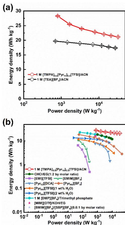
Fig. 7 Ragone plots of activated carbon supercapacitors: (a) BILs electrolyte (1 M [TMPA]<sub>0.5</sub>[Py<sub>14</sub>]<sub>0.5</sub>[TFSI]/ACN) and commercial organic electrolyte (1 M [TEA][BF<sub>4</sub>]/ACN); (b) BILs electrolyte and ILs electrolytes.
