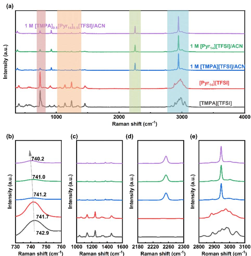
Fig. 3 Raman spectra of hybrid electrolytes in different frequency ranges: (a)  $50\text{--}4000 \text{ cm}^{-1}$ , (b)  $730\text{--}760 \text{ cm}^{-1}$ , (c)  $1000\text{--}1600 \text{ cm}^{-1}$ , (d)  $2180\text{--}2300 \text{ cm}^{-1}$ , and (e)  $2800\text{--}3100 \text{ cm}^{-1}$ .
