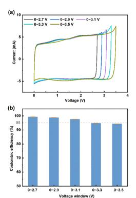
Fig. 5 (a) CV curves and (b) coulombic efficiency of 1 M [TMPA] $_{0.5}$ [-Pyr $_{14}$ ] $_{0.5}$ [TFSI]/ACN at different cut-off voltages.
