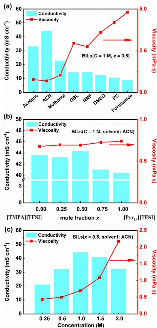
Fig. 2 Conductivity and viscosity of hybrid electrolytes at different (a) solvents, (b) cationic types and proportions, and (c) concentrations. In which, mole fraction  $x = n([\text{Pyr}_{14}^{+}]) : n([\text{TMPA}^{+}])$ .
