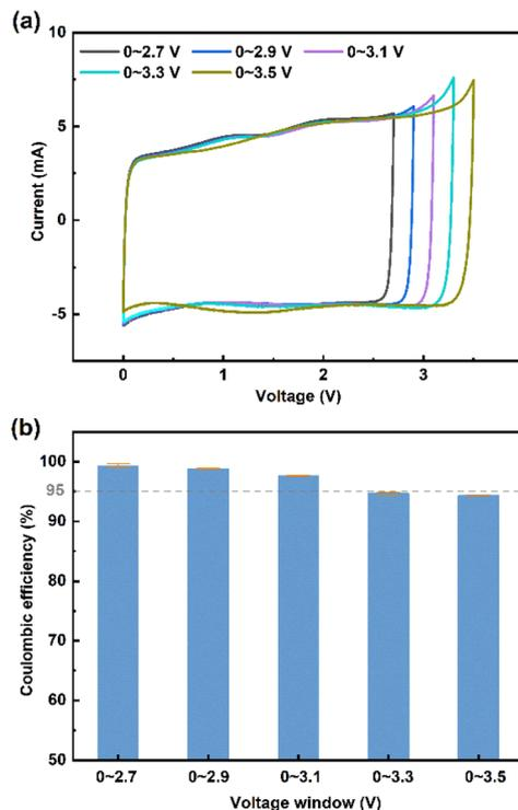
Fig. 5 (a) CV curves and (b) coulombic efficiency of 1 M [TMPA]<sub>0.5</sub>[-Pyr<sub>14</sub>]<sub>0.5</sub>[TFSI]/ACN at different cut-off voltages.
