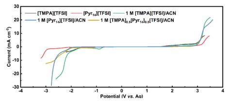
Fig. 4 Linear sweep voltammetry curves of various electrolytes.
