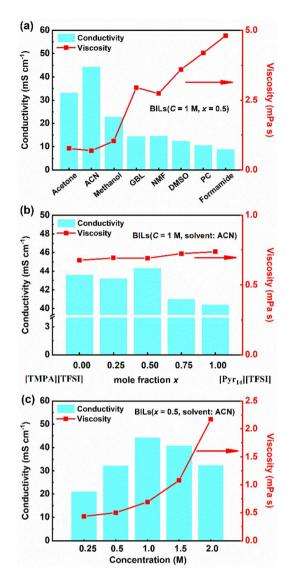
Fig. 2 Conductivity and viscosity of hybrid electrolytes at different (a) solvents, (b) cationic types and proportions, and (c) concentrations. In which, mole fraction  $x = n([Pyr_{14}^+]) : n([TMPA^+])$
