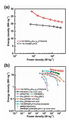
Fig. 7 Ragone plots of activated carbon supercapacitors: (a) BILs electrolyte (1 M [TMPA] $_{0.5}$ [Pyr $_{14}$ I $_{0.5}$ [TFSI]/ACN) and commercial organic electrolyte (1 M [TEA][BF $_4$ ]/ACN); (b) BILs electrolyte and ILs electrolytes.
