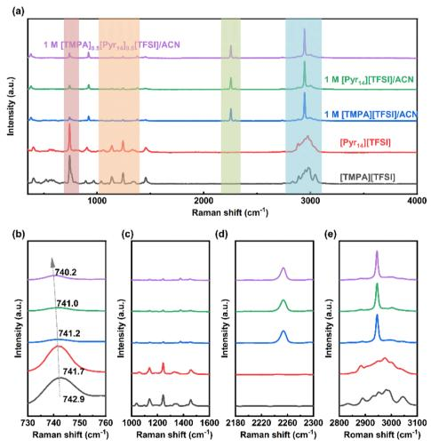
Fig. 3 Raman spectra of hybrid electrolytes in different frequency ranges: (a)  $50-4000 \, \mathrm{cm}^{-1}$ , (b)  $730-760 \, \mathrm{cm}^{-1}$ , (c)  $1000-1600 \, \mathrm{cm}^{-1}$ , (d)  $2180-2300 \, \mathrm{cm}^{-1}$ , and (e)  $2800-3100 \, \mathrm{cm}^{-1}$ .
