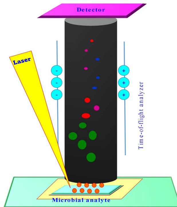
Fig. 1 Schematic showing components of MALDI-TOF MS.
