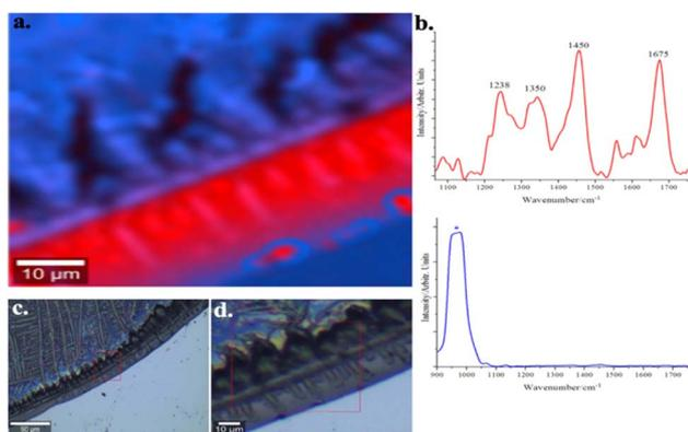
Fig. 2 (a) Raman image of the coffee-ring formed with mabIL-6 on Si/SiO<sub>2</sub>, (b) the red Raman spectrum corresponds to the mabIL-6 and the blue one to the Si/SiO<sub>2</sub>; (c) and (d) optical images of the coffee-ring, the region where the image was taken is shown in the red box.
