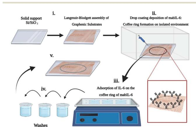
Scheme 1 Scheme shows (i) Langmuir-Blodgett (LB) assembly of graphene substrates (rGO-NH<sub>2</sub> and GO) on solid support, (ii) drop coating deposition of mabIL-6 (coffee-ring formation) on LB thin films of graphenic substrates, (iii) adsorption of IL-6 on the coffee-ring of mabIL-6, (iv) series of washes of the arrays, (v) Si/SiO<sub>2</sub>/graphenic substrates/mabIL-6/IL-6 arrays for Raman measurements. Created with <https://BioRender.com>.
