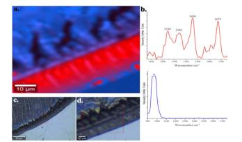
Fig. 2 (a) Raman image of the coffee-ring formed with mabIL-6 on Si/ SiO<sub>2</sub>, (b) the red Raman spectrum corresponds to the mabIL-6 and the blue one to the Si/SiO<sub>2</sub>; (c) and (d) optical images of the coffee-ring, the region where the image was taken is shown in the red box.
