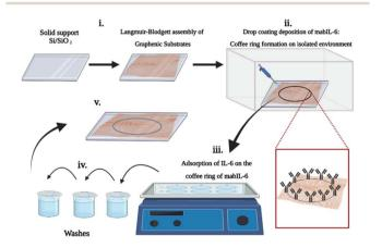
Scheme 1 Scheme shows (i) Langmuir-Blodgett (LB) assembly of graphene substrates (rGO-NH<sub>2</sub> and GO) on solid support, (ii) drop coating deposition of mabIL-6 (coffee-ring formation) on LB thin films of graphenic substrates, (iii) adsorption of IL-6 on the coffee-ring of mablL-6, (iv) series of washes of the arrays, (v) Si/SiO<sub>2</sub>/graphenic substrates/mabIL-6/IL-6 arrays for Raman measurements. Created with https://BioRender.com.
