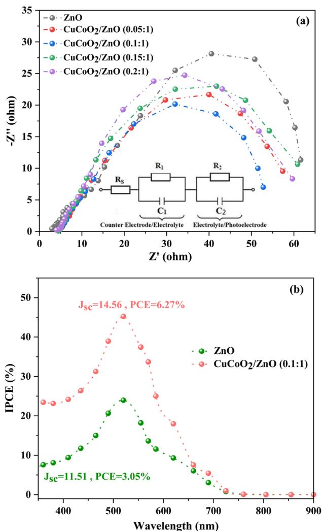
Fig. 12 (a) The Nyquist diagrams of all solar cells assembled with ZnO and  $\text{ZnO}/\text{CuCoO}_2$  photoelectrodes. (b) IPCE spectra of DSSCs based on ZnO and  $\text{CuCoO}_2/\text{ZnO}$  (0.1 : 1) photoelectrodes.
