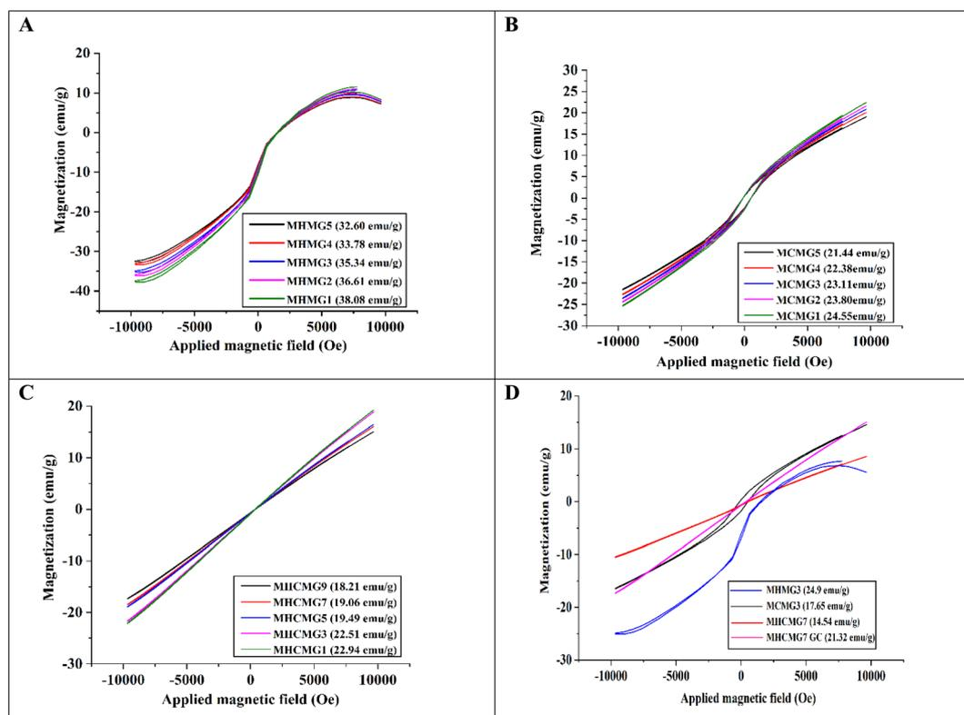
Fig. 2 VSM analyses of different MM (A) HNTs/ $\text{Fe}_3\text{O}_4$  (MHMG1 to MHMG5), (B) CTS/ $\text{Fe}_3\text{O}_4$  (MCMG1 to MCMG5) (C) CTS/ $\text{Fe}_3\text{O}_4$ /HNTs (MHCMG1 to MHCMG9), and (D) comparative VSM analysis of optimized formulation MCMG3, MHMG3, MHCMG7 and MHCMG7 GC (gemcitabine loaded) microspheres.
