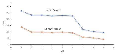
Fig. 5 Validity of pH on the implementation of the investigated electrode.
