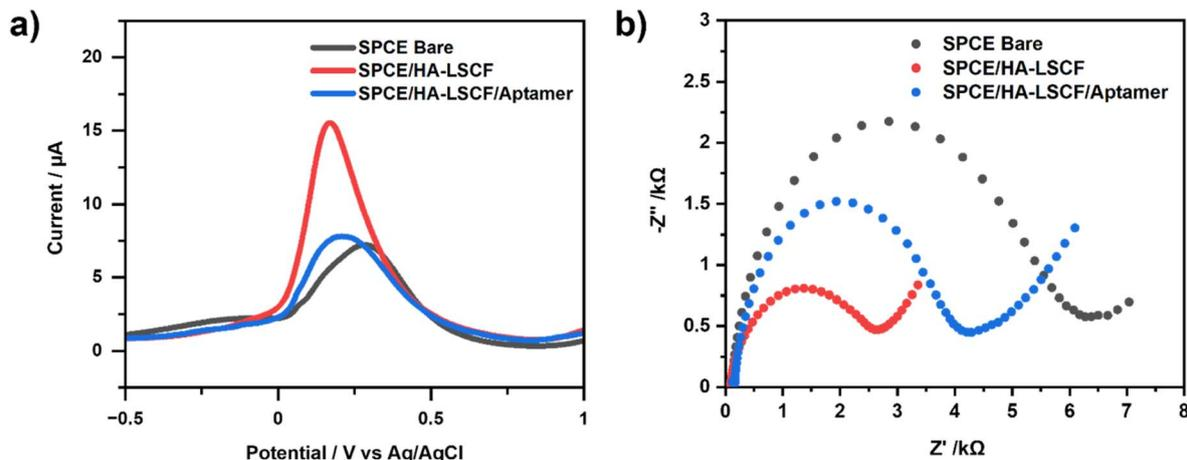
Fig. 4 Electrochemical characterization results (a) voltammogram  $[\text{Fe}(\text{CN})_6]^{3-/4-}$  10 mM in 0.1 M KCl over a potential range of  $-0.5$  to  $+1.0$  V with a scan rate of  $0.008 \text{ V s}^{-1}$  at SPCE bare, SPCE/HA-LSCF, and SPCE/HA-LSCF/apptamer. (b) Nyquist plots of  $[\text{Fe}(\text{CN})_6]^{3-/4-}$  10 mM in 0.1 M KCl on SPCE bare, SPCE/HA-LSCF, and SPCE/HA-LSCF/apptamer.
