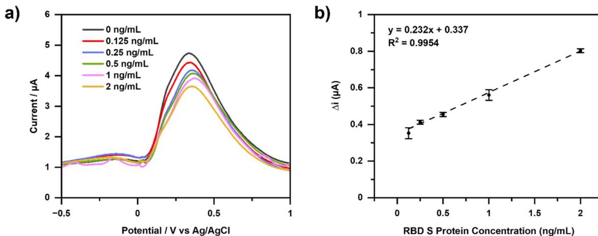
Fig. 5 Electrochemical characterization results (a) voltammogram of various RBD S protein concentrations (0, 0.125, 0.25, 0.5, 1.0, 2.0 ng mL<sup>-1</sup>), with the redox system [Fe(CN)<sub>6</sub>]<sup>3-/4-</sup> 10 mM in KCl 0, 1 M uses DPV over a potential range of -0.5 V to +1.0 V with a scan rate of 0.008 V s<sup>-1</sup>. (b) Calibration curve of variation of RBD spike protein concentration.
