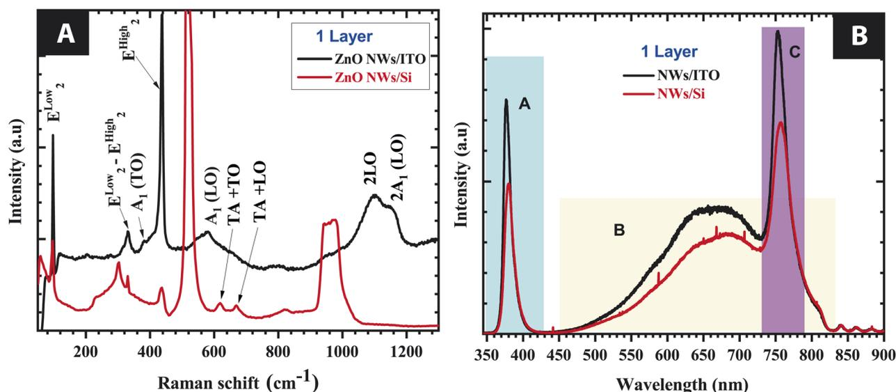
**Fig. 4** (A) Raman spectra, and (B) PL spectra of ZnO NFs grown on an ITO and Si substrate with 100 nm-thick of ZnO sol-gel thin film used as buffer layer.
