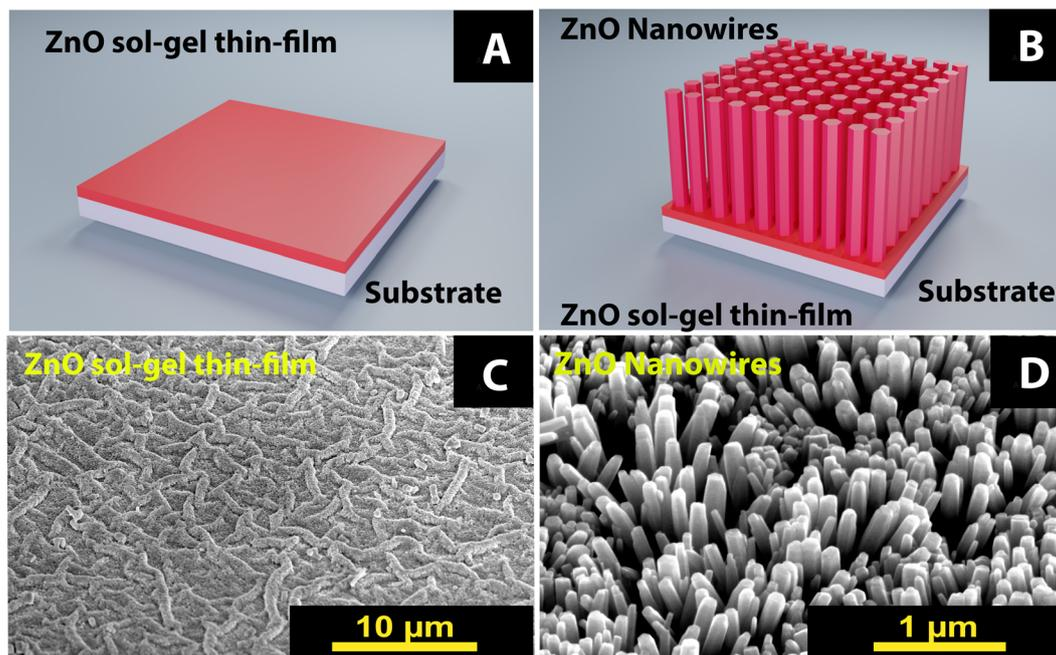
Fig. 1 Schematic representation of the steps fabrication based on a combination of sol–gel synthesis and chemical bath deposition process of ZnO nanowires (A) on ZnO sol–gel thin-film deposited on substrate by spin coating, (B) ZnO nanowires arrays. (C) and (D), SEM images of the as-grown ZnO nanowire arrays on the substrate (C), ZnO sol–gel thin-film after spin-coating, and (D) ZnO nanowires grown.
