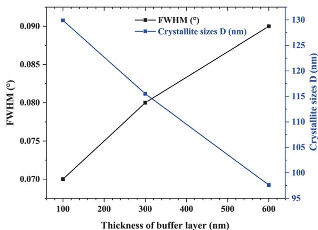
Fig. 7 FWHM and crystallite size of the ZnO NWs as a function of buffer layer thickness.
