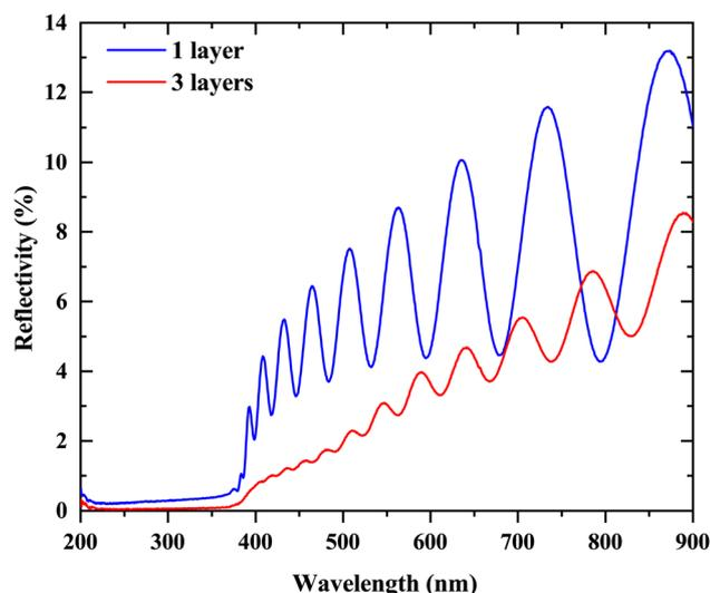
Fig. 8 The reflectivity spectrum of ZnO NWs grown on a Si substrate with one buffer layer and 3 buffer layers.
