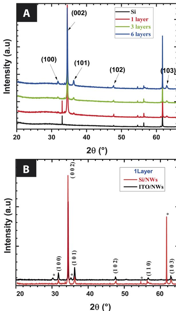
Fig. 6 XRD pattern of ZnO NWs growth (A) on silicon substrate covering with buffer layer of varying thickness, and (B) on ITO substrate with one buffer layer (100 nm thick).
