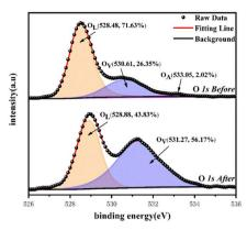
Fig. 6 XPS curves for O 1s of the original and tested YSZ $-CeO_2$  (70 : 30, wt/wt) electrolyte.
