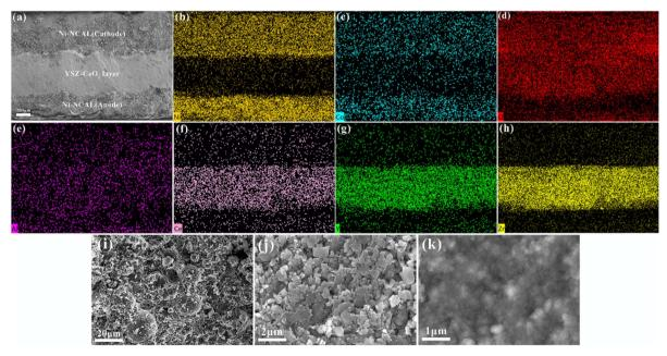
Fig. 3 (a) Cross-sectional SEM images of the tested fuel cell with YSZ-CeO<sub>2</sub> (70:30, wt/wt) electrolyte, (b)-(h) EDS mappings of the tested fuel cell from the cross-sectional view, magnified SEM images of (i) cathode region, (j) anode region, and (k) detailed morphology of the YSZ-CeO<sub>2</sub> (70:30, wt/wt) electrolyte membrane.
