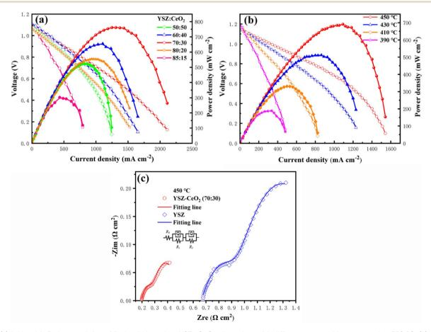
Fig. 2 (a) I-V and I-P characteristics of fuel cells based on YSZ-CeO<sub>2</sub> electrolyte with different composition operated at 550 °C; (b) electrochemical performance of YSZ-CeO<sub>2</sub> (70:30, wt/wt) based SOFC measured at 450 °C-390 °C; (c) EIS curves of SOFC with YSZ-CeO<sub>2</sub> (70:30, wt/wt) electrolyte and SOFC with YSZ electrolyte under 450 °C (dots for experimental data; line for fitting data). H<sub>2</sub> and air were adopted as fuel and oxidant, respectively.
