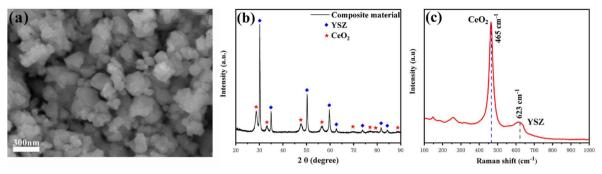
Fig. 1 (a) The SEM images of the as-prepared YSZ- $CeO_2$  (70:30) powders, (b) the XRD patterns of YSZ- $CeO_2$  (70:30) and (c) Raman spectrum of hydrogen treated YSZ- $CeO_2$  (70:30) powder.
