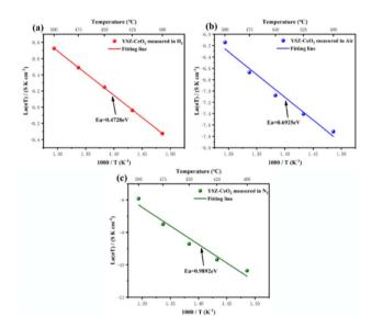
Fig. 5 Arrhenius curves of the original YSZ-CeO<sub>2</sub> electrolyte obtained in different atmospheres: (a) H<sub>2</sub>, (b) air and (c) N<sub>2</sub>.
