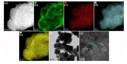
Fig. 4 (a) TEM and corresponding EDS images of (b) Ce, (c) Y, (d) Zr and (e) O elements, (f and g) HR-TEM images of the tested YSZ-CeO<sub>2</sub> electrolyte.
